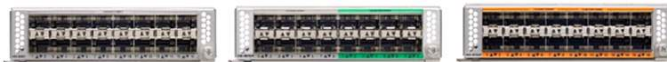
Figure 4. From Left to Right: 16-Port 1 and 10 Gigabit Ethernet and FCoE Module, 8-Port Fibre Channel Plus 8-Port 1 and 10 Gigabit Ethernet and FCoE Module, and Unified Port Module
