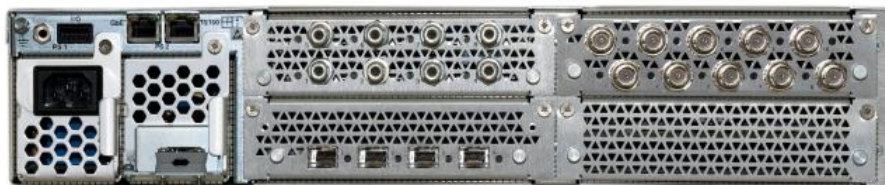
Figure 2. Cisco DCM Series D9900 Transcoder Rear Panel with AC and DC power supply, 1 GbE card, and 3 Transcoder cards
