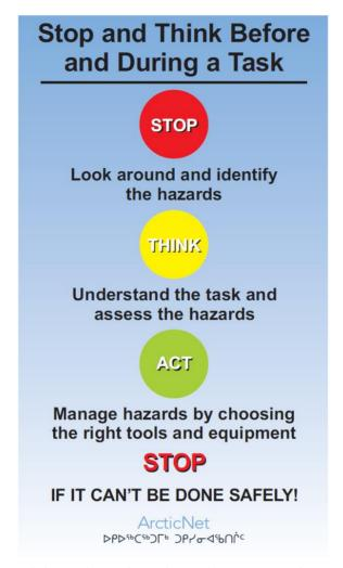
Figure 1 Stop and Think cards provided to workers and posted in work areas as reminders to assess safety and identify hazards during operations.
