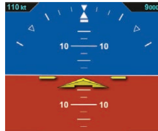
Figure 4-10 Airspeed Tape Disabled
