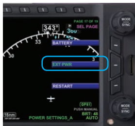
Figure 6-3 External Power Voltage Status
