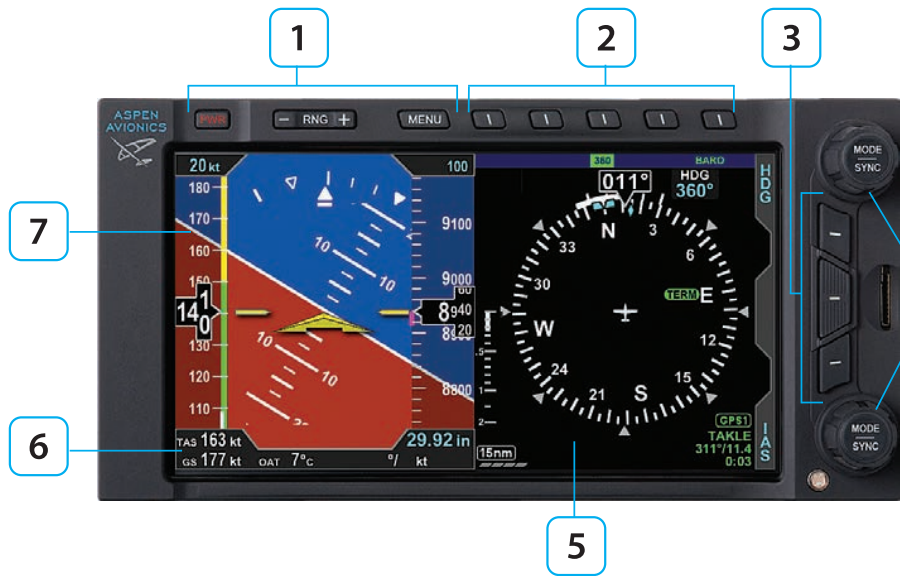
Figure 1 Evolution Backup Display – Basic, Landscape Version – Knobs, Buttons, and Keys
