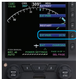
Figure 6-3 External Power Voltage Status
