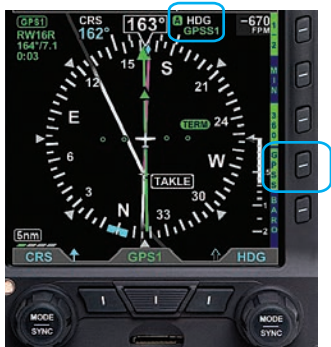
Figure 6-9 Operating in GPSS Mode
