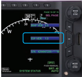
Figure 7-2 View Input/Output Processor Software Version
