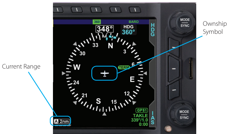
Figure 3-15 Current Range 2nm from Ownship to Edge of Compass Rose
