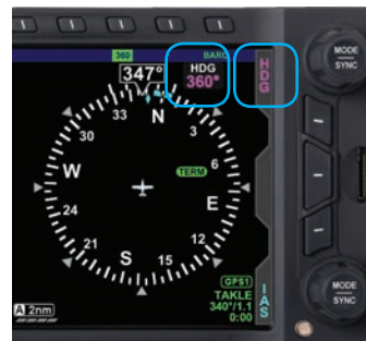
Figure 3-8 Selected Heading Field Enabled
