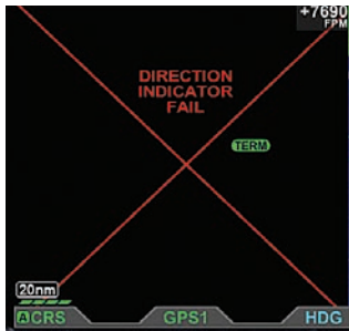
Figure 4-86 Direction Indicator Fail
