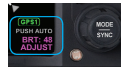
Figure 5-28 Display Brightness in BRT ADJUST Mode
