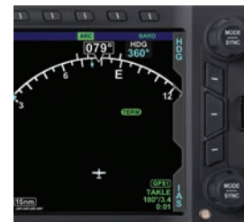
Figure 4-83 Selected Heading Bug Outside of the ARC Compass Scale Range
