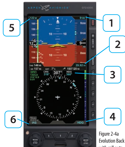
Figure 2-4 Bottom and Top Knobs and Corresponding Fields
