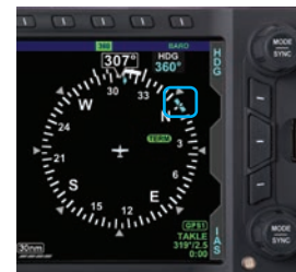
Figure 4-82 Heading Bug and Selected Heading Field
