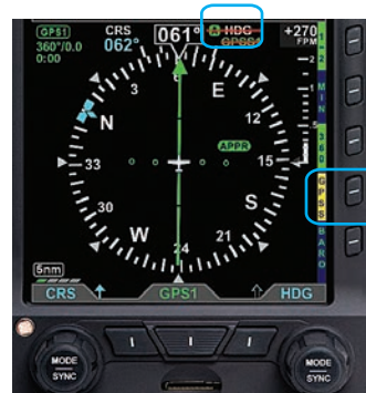
Figure 6-10 GPSS in Wings Level Mode
