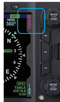
Figure 4-21 BARO Field Enabled
