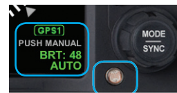
Figure 5-27 Display Brightness in BRT AUTO Mode
