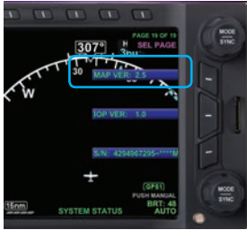
Figure 7-1 View Main Application Processor Software Version
