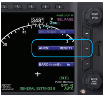
Figure 6-7 AHRS Reset Menu Key
