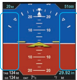
Figure 4-35 Airspeed and Altitude Tape Disabled
