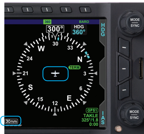
Figure 3-16 Current Range 30nm from Ownship to Edge of Compass Rose
