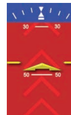
Figure 4-5 Pitch Markings Large Pitch Up
