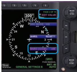
Figure 4-20 BARO Set to mB (millibars)
