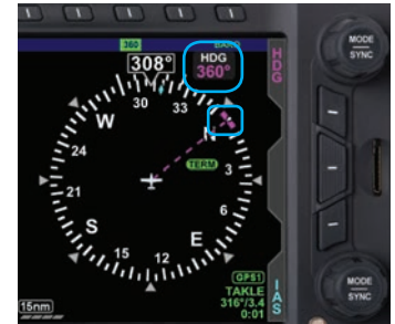
Figure 2-6 HDG field updated and inactive
