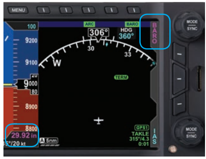
Figure 3-6 BARO Setting Field Enabled
