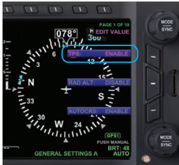
Figure 4-9 Editing Airspeed Tape Display
