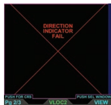
Figure 6-12 Direction Indicator Fail
