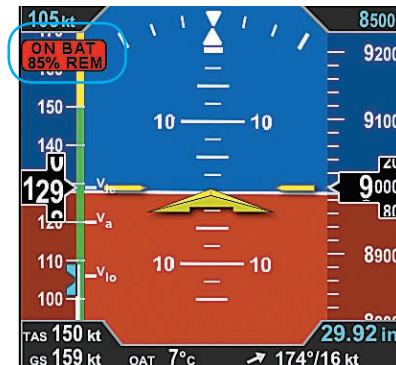
Figure 6-2 Battery Charge Remaining
