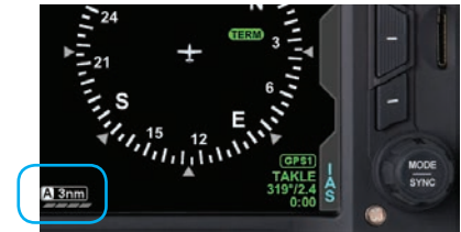
Figure 2-29 Map in ARC Compass Mode, 3nm Range at Declutter Level 0
