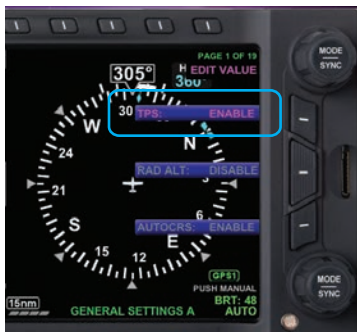
Figure 4-34 Editing Airspeed and Altitude Tape Display
