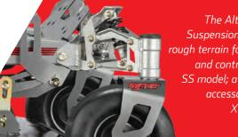
The Altoz Independent Front Suspension (IFS) smooths out rough terrain for superb comfort and control. Standard on SS model; available as an accessory on other XE models.
