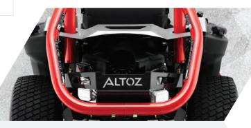
Our roll-over protection system can be folded down easily to avoid low hanging limbs.
