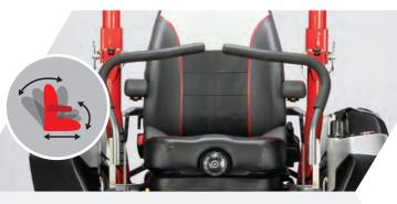
Combined with our suspension system, the 12-way adjustable high-back suspension seat with arm rests delivers the industry's smoothest ride.
