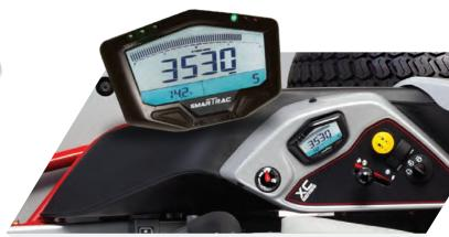
SmarTrac™ Monitoring System features a tachometer and resettable hour meter, with alerts for low oil pressure and overheating.
