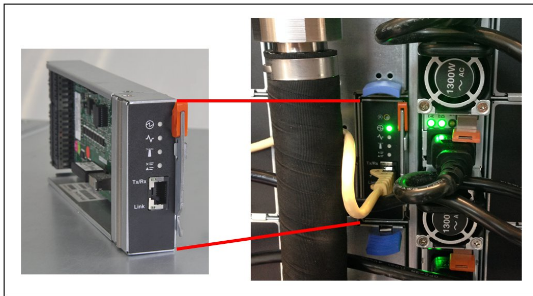
Figure 16. Fan and Power Controller
