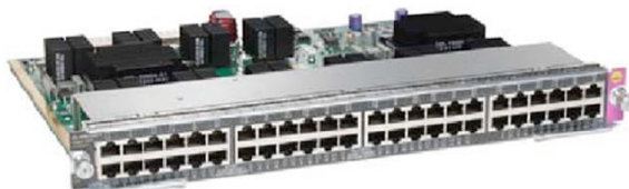
Figure 12. WS-X4748-UPOE+E Cisco Catalyst 4500E Series 48-Port 802.3af PoE, 802.3at PoEP, and UPOE 10/100/1000 (RJ-45)
