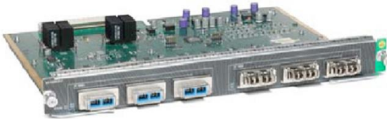
Figure 4. WS-X4606-X2-E Cisco Catalyst 4500E Series 6-Port 10 Gigabit Ethernet (X2)
