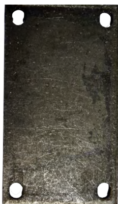
BPR07 Base plate size: 177 x 100 Hole centres: 152 x 76 Suits bolt size: 10mm Series: 500 + 1000
