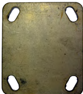
BPR04 Base plate size: 114 x 100 Hole centres: 76 x 67/92 x 76 Suits bolt size: 3/8 Series: Heavy Industrial
