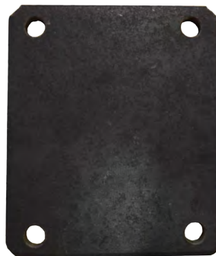
BPR04 Base plate size: 114 x 100 Hole centres: 76 x 67/92 x 76 Suits bolt size: 3/8 Series: Heavy Industrial
