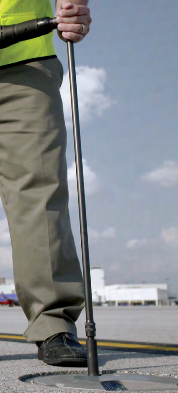
Data about torquing of in-pavement lights is transmitted via Wi-Fi for tracking and analysis.
