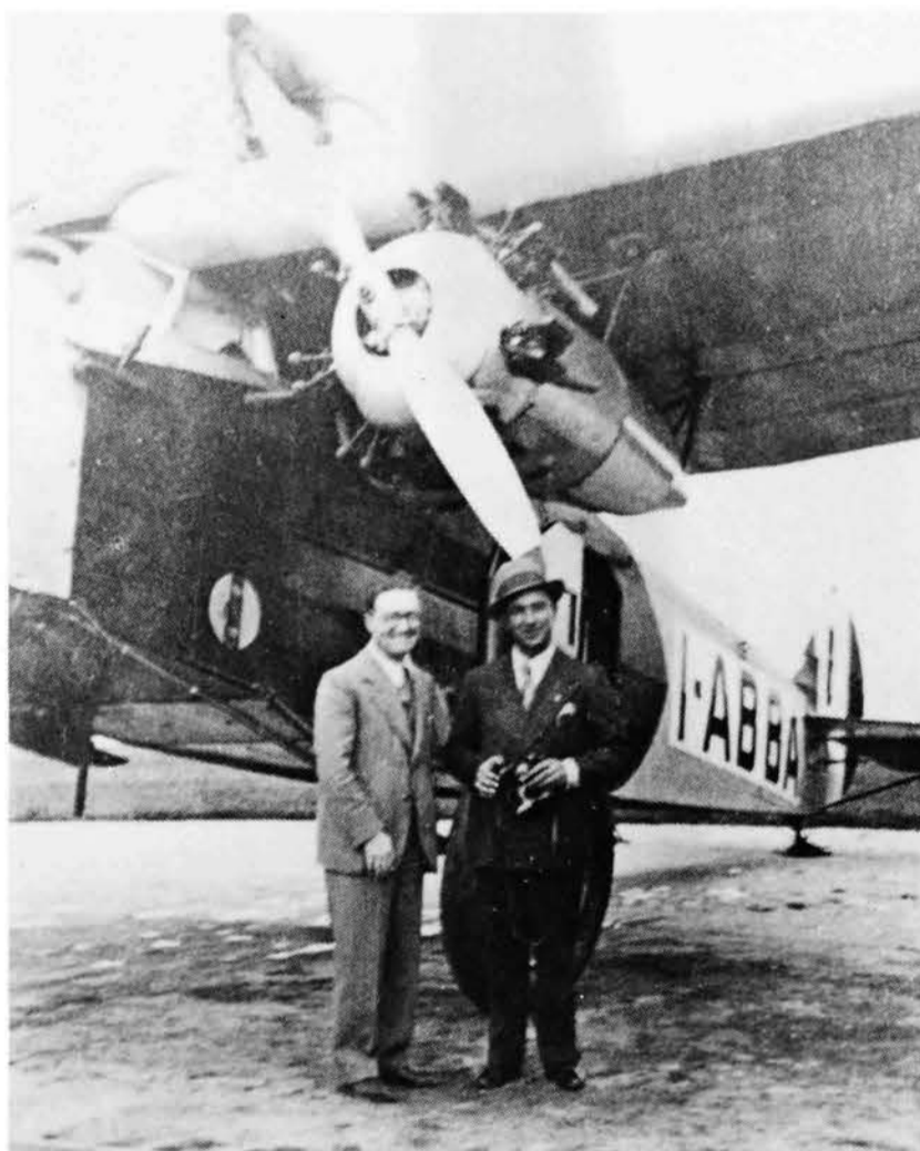
Above: Avio Linee Italiane I-ABBA c/n 5212 receives some attention on top while would-be passengers pose for the camera below. Note the close cowling covering all but the cylinder heads and stub exhausts of the Lynx engine. (Roberto Gentilli)
