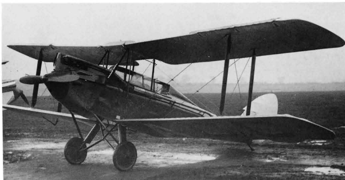
Right: W. R. Bailey's G-AADC is here seen to be a standard coupé Moth with the old standard wide tyres and long exhaust pipe. The wing-folding notice can be seen in the normal position by the leading edge wing root. (via Jack Meaden)
