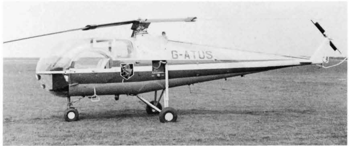
Above: G-ATUS c/n 1030 seen during May 1968 when owned by the Quinton Hazell company and based at Colwyn Bay, hence the prominent Welsh Dragon badge. The square opening ahead of the undercarriage strut is for access to, and exhaust from, the Lycoming IVO-540 engine. (R.W.Simpson via Peter Keating)
