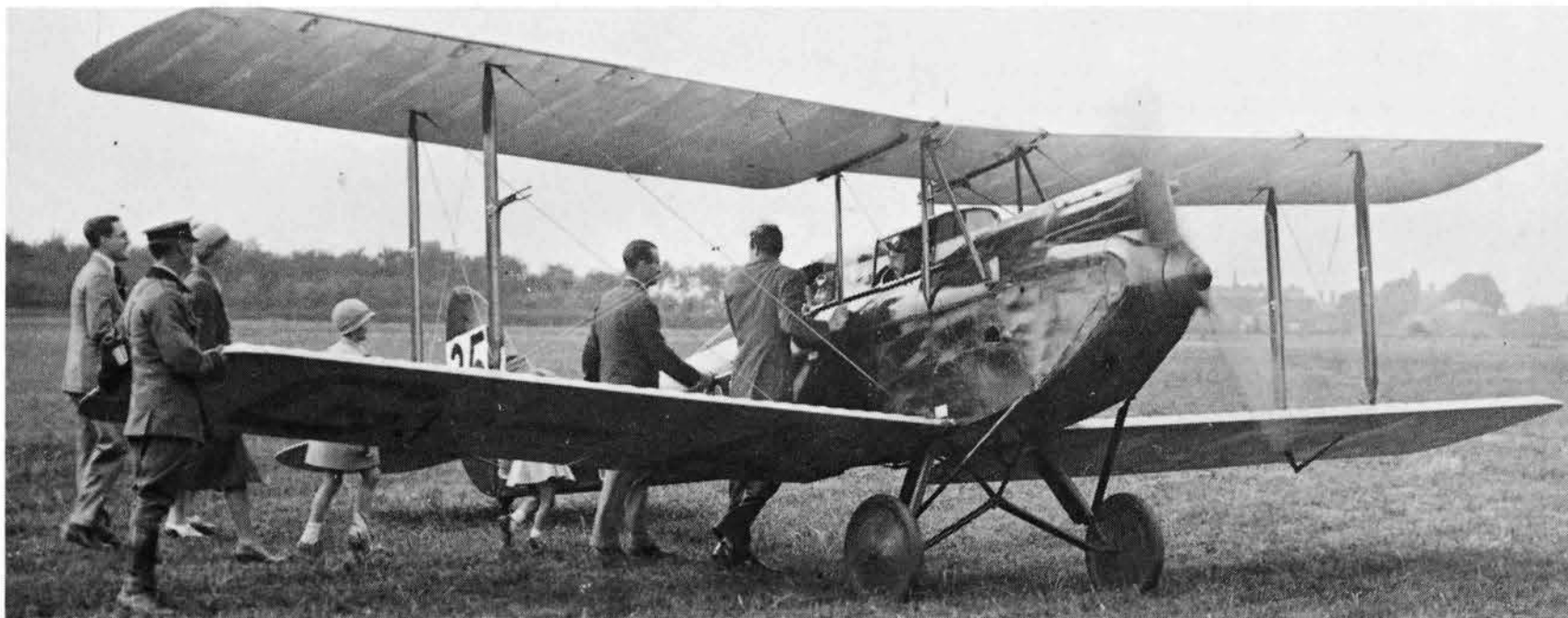
Above: Alan Butler's G-AACL wearing racing number 25. It was a standard coupé Moth with the newly-introduced slim wheels and narrower tyres. These became popular with private owners until doughnut tyres became available in 1931. (Aeroplane via Jack Meaden)
