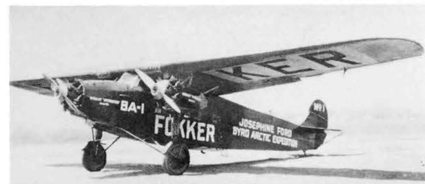
Above: The first aircraft to fly over the North Pole was the first F.VIIa/3m trimotor "Josephine Ford" flown by Cdr Richard Byrd. Originally designed for the 1925 Ford Reliability Tour which it won, c/n 4900 was an F.VIIa conversion fitted with three 200 hp 9 cylinder Wright J4B radial engines. (via Jack Meaden)
