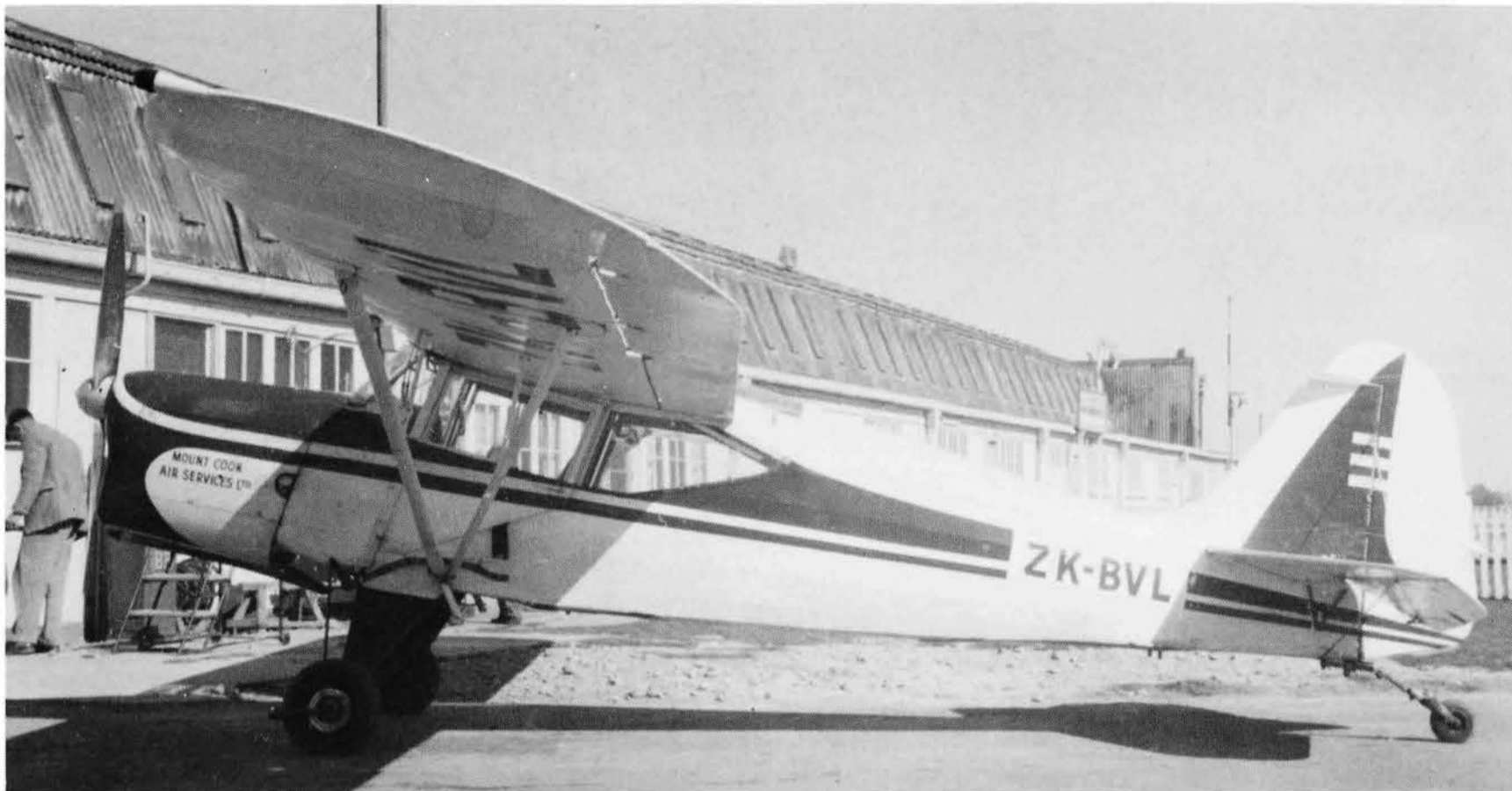
Above: Auster Autocar ZK-BVL of Mount Cook Air Services at Christchurch. A long lever is fitted below the pilot's door and is connected to the undercarriage in such a way as to suggest that it could be used to "jack" the aircraft up for skis to be fitted or removed easily. Alternative suggestions would be welcome!
