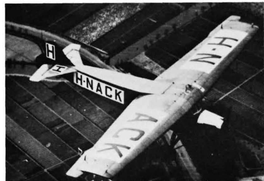
Above: The prototype F-VII c/n 4759 H-NACC with 360 hp 12 cylinder vee water-cooled Rolls Royce Eagle IX. Notable are the balanced "elephant ear" ailerons and the oval rudder, larger than the rudder fitted on early flights. Only five F-VII aircraft were built. (via Jack Meaden) Below: A view of the third F.VII c/n 4840 H-NACK in flight with the distinctive shape of the ailerons again clearly visible. (via Harm Hazewinkel)
