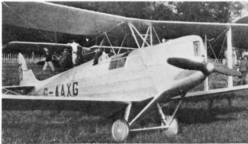
Left: Two views of G-AAXG showing the redesigned centre section struts to allow access to the enclosed front cockpit and the closely-cowled Gipsy engine.
