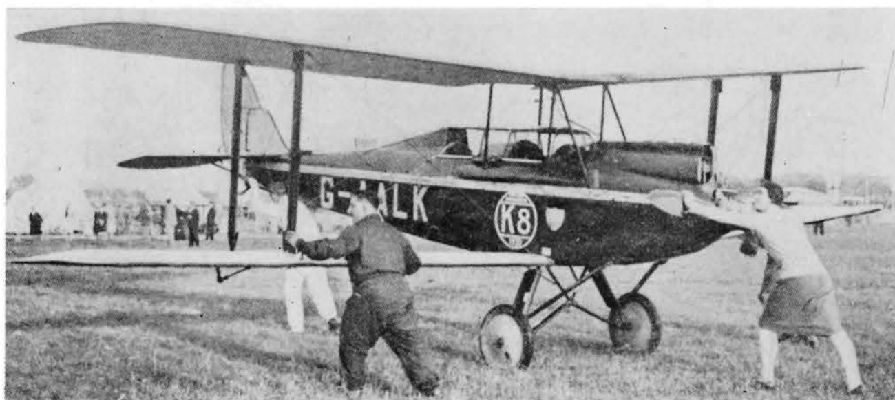
Above: DH.60M G-AAGE as coupé demonstrator with "Gipsy Moth" on the fuselage sides, a characteristic of DH Company Moths (see p.90/79). Here 'GE' is returning from Teignmouth while located at Filton. Right: Miss Winifred Spooner has help to move G-AALK as "K8" in the 1930 Challenge Internationale de Tourisme. Lifting the tail by the tailplane bracing strut allowed one person to move the Moth, but on rough ground help was needed to push. (both Aeroplane via J.M.)
