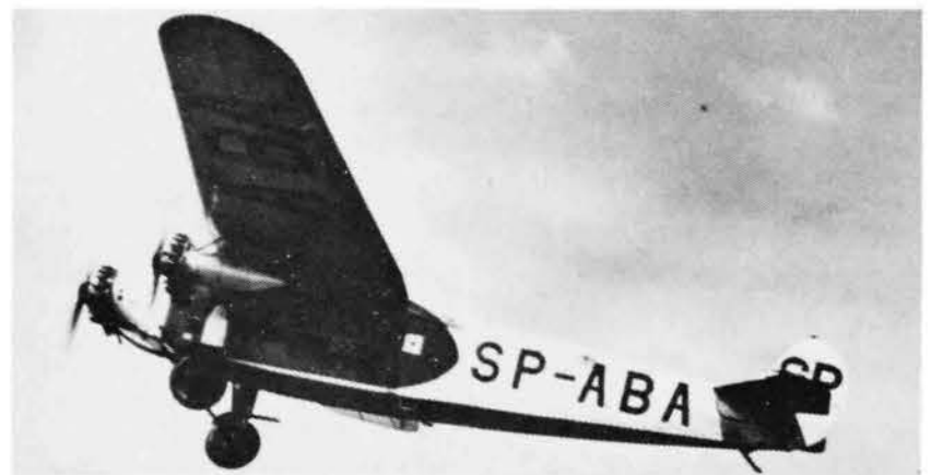
Above: F.VIIb/3m SP-ABA "Anka" c/n 1 climbing out after take-off. The relatively small fin and rudder was considered adequate throughout the life of the type, although Kingsford Smith had a larger rudder fitted after his early flights on "Southern Cross", no doubt after trying the effects of shutting down a wing engine. (via J.M.)
