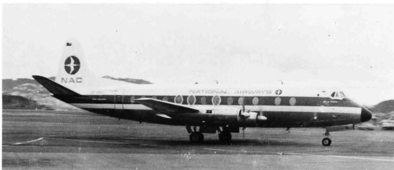
Above: National Airways V.807 Viscount ZK-BWO "City of Dunedin" taxiing on inboard engine power. (R.W.Kerr)
