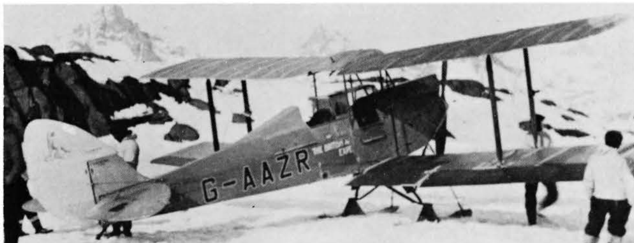
Right: Coupé G-AAZR on skis with polar bear painted on the rudder and "The British Arctic Air Route Expedition" on the fuselage. This photo shows well how the downward-opening door flap was needed on the front cockpit to allow the occupant to get in and out. The roof has been removed from the pilot's (rear) cockpit and the wing-folding jury struts are in position. (via Jack Meaden)
