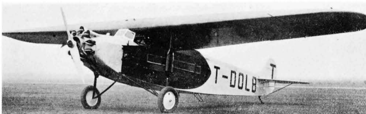
Left: F.VIIa c/n 5058 T-DOLB of Denmark's DDL with a 450 hp Jupiter VI. The direct drive Jupiter was fitted with a left hand tractor fixed pitch propeller, in this case the twisted metal Fairey-Reed type. (Aeroplane via Jack Meaden) Far left: H-NAFA c/n 5069, marked FVII 3M, before it became PK-AFA in the East Indies. (via H.Hazewinkel)
