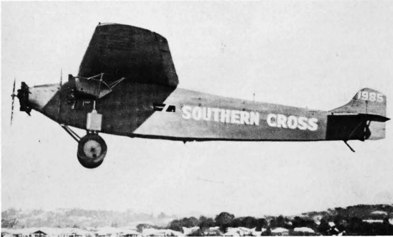
Left: Originally F-VIIa/3m "Detroit" with 200 hp Wright J4B engines, c/n 4954 was fitted with the long span wing and 220 hp Wright J5C engines to become 1985 "Southern Cross" in which Charles Kingsford Smith was the first to fly the Pacific Ocean, from Oakland to Brisbane between 31.5.28 and 9.6.28. Showing the larger squared-off rudder fitted earlier, 1985 is seen here taking off from Brisbane for Sydney after completing the Trans-Pacific flight. (Aeroplane via Jack Meaden)
