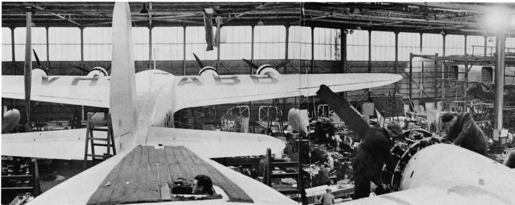
Above: "Coolangatta" which crashed on 11.10.44 is seen here at Short's being prepared for Qantas as VH-ABB. Power units were four Bristol Pegasus Xc 9-cylinder radials giving 740 rated hp, 920 hp for takeoff. Originally G-AFBK, it became A18-13 with the RAAF in 9.39 serving with 11 and 41 Squadrons before returning to Qantas as VH-ABB on 13.7.43. (Aeroplane, via Jack Meaden)
