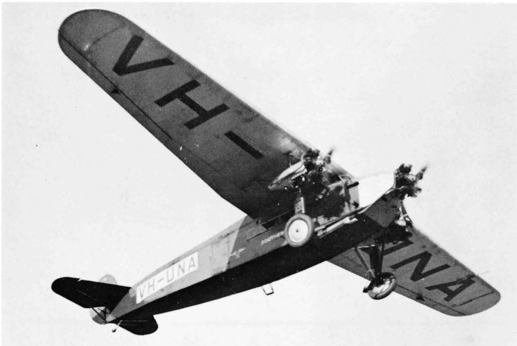
Above: Avro Ten c/n 388 VH-UNA "Southern Sun" flies over in a revealing shot from a seldom-seen angle which clearly shows the straight centre section of the wing between the engines introduced on the F.VIIb variants. (via Jack Meaden) Below: Late production Avro Ten c/n 527 G-ACGF was supplied to Midland & Scottish Air Ferries. The F.VIIb/3m was an aircraft from the days of grass airfields and tailskids, but Avro Tens c/n 524 to 527 were exceptions in each having a tailwheel fitted as seen here on G-ACGF. (Aeroplane via Jack Meaden)
