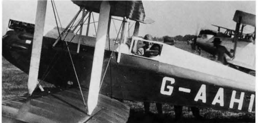
Above: Nigel Norman's G-AAHI flew in the 1930 King's Cup as a single-seater with a hood over the pilot's cockpit faired right back to the tail and with the front cockpit covered over. It also had stub exhausts fitted. (via Jack Meaden)
