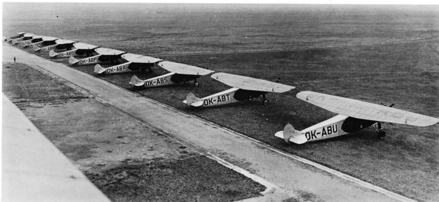
Above: Ten F.VIIb/3m aircraft of Ceskoslovenska Letecka Spolecnost (C.L.S.) lined up at Kbely aerodrome near Prague, Czechoslovakia, with an Avia BH25 at the end. The eight nearest aircraft are Avia-built with 240 hp Walter "Castor" engines and 3-blade propellers. (via Jack Meaden)
