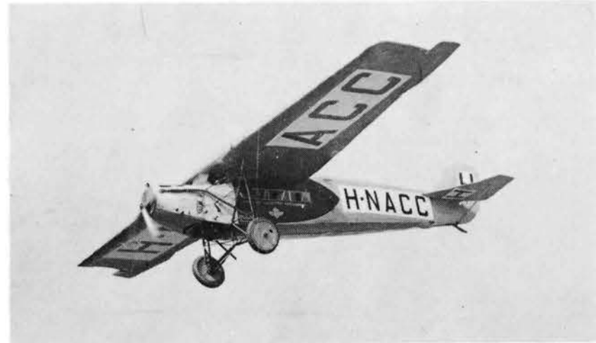
Above: The prototype F-VII c/n 4759 H-NACC with 360 hp 12 cylinder vee water-cooled Rolls Royce Eagle IX. Notable are the balanced "elephant ear" ailerons and the oval rudder, larger than the rudder fitted on early flights. Only five F-VII aircraft were built. (via Jack Meaden) Below: A view of the third F.VII c/n 4840 H-NACK in flight with the distinctive shape of the ailerons again clearly visible. (via Harm Hazewinkel)
