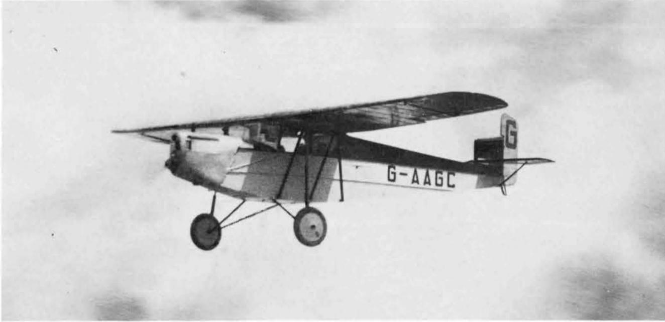
Left: G-AAGC was the second Koolhoven FK.41. It was brought to the UK to become the first Desoutter I, in which form the tailplane was lowered from the top of the fin to the top of the fuselage and changes were made to the cowlings to suit a 105 hp Hermes engine as seen here. (Jack Meaden)
