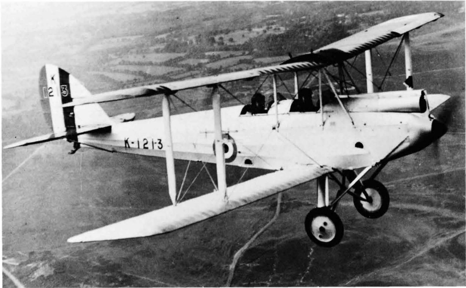
Above: DH.60M Moth K1213 c/n 1525, with fuselage stringers and upper leading-edge slots clearly visible, was delivered to the CFS in 1930 which is presumably when this manufacturer's photograph was taken. (BAe via Mike Hooks)
