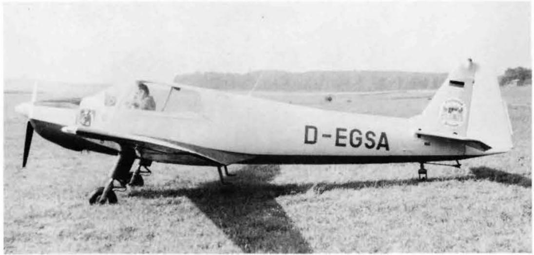
The next development was the 4-seat K1 107D using a Lycoming O-360-ALA engine, with a redesigned Piper Comanche-like canopy to reduce cockpit noise levels, and a larger tail. C/n 145 was initially chosen as the prototype but a new c/n series beginning 201 was defined in 7.60 and the marks D-EGSA reserved for the K1 107D V-1 on 14.7.60.
