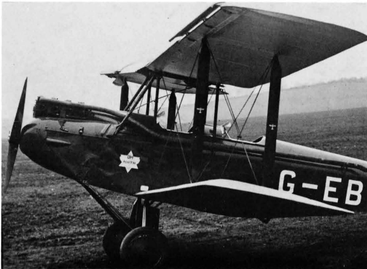
Left: G-EBTD before the slot demonstration accident. The open slats show the cutaway wing leading edge of the initial installations and on the right side a slat-angle quadrant is fitted to this experimental application. The Gipsy left-side carburettor and exhaust manifold can be seen and below them the carburettor intake added to the modified Cirrus-type cowling. (via Jack Meaden)
