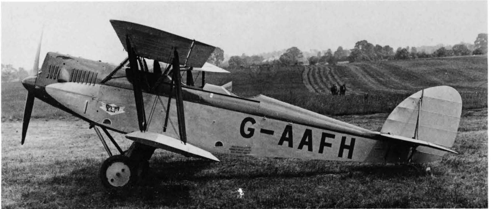
Above: Prototype Parnall Elf G-AAFH c/n 1 pushed out at Yate to be photographed after painting. Structure was mostly wood with ply box fuselage and fabric covered wings which could be folded to a width of 7ft 11in. The 105 hp Hermes 4-cyl upright in-line engine was completely cowled, fuel from the 20-gal fuselage tank being pumped up to the 3-gal gravity tank in the slim centre section of the top wing. (Via Jack Meaden)
