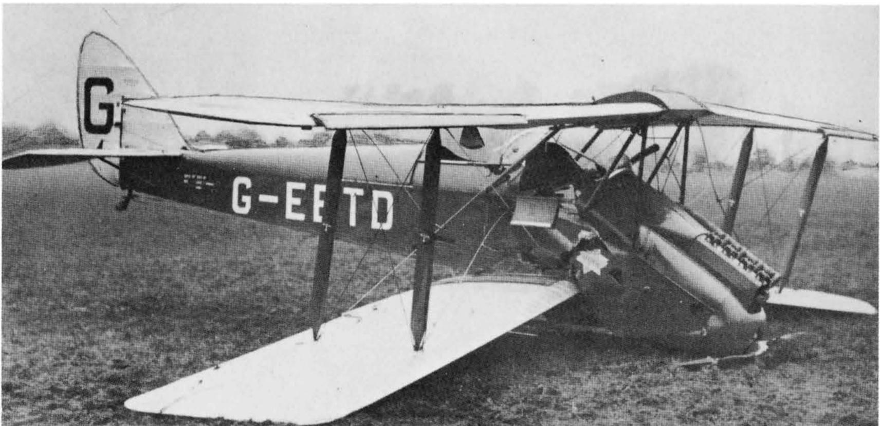
stalling speed of the DH.60G without slots was quoted by the maker as 44 mph. The writer made a check on the stall of a DH.60G with slots and recorded it as 39-40 mph, so slots reduced the stalling speed of the Moth by 4 or 5 mph under approach conditions and of course also promoted recovery at a lower speed and so reduced the likelihood of a spin.
