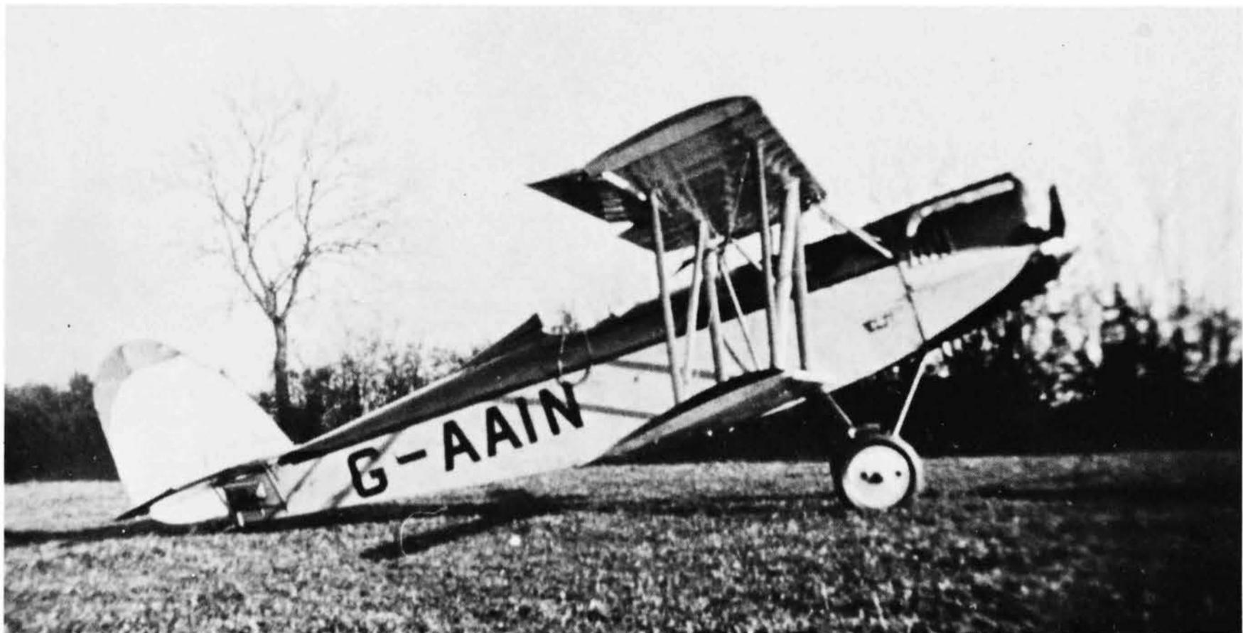
Above: Lord Apsley's Parnall Elf 2 G-AAIN, which differed from the Mk 1 (see page 90/11) in having the horn-balanced rudder, seen here in a field near Tetbury, Gloucestershire in the winter of 1938-9. (Jack Meaden)
