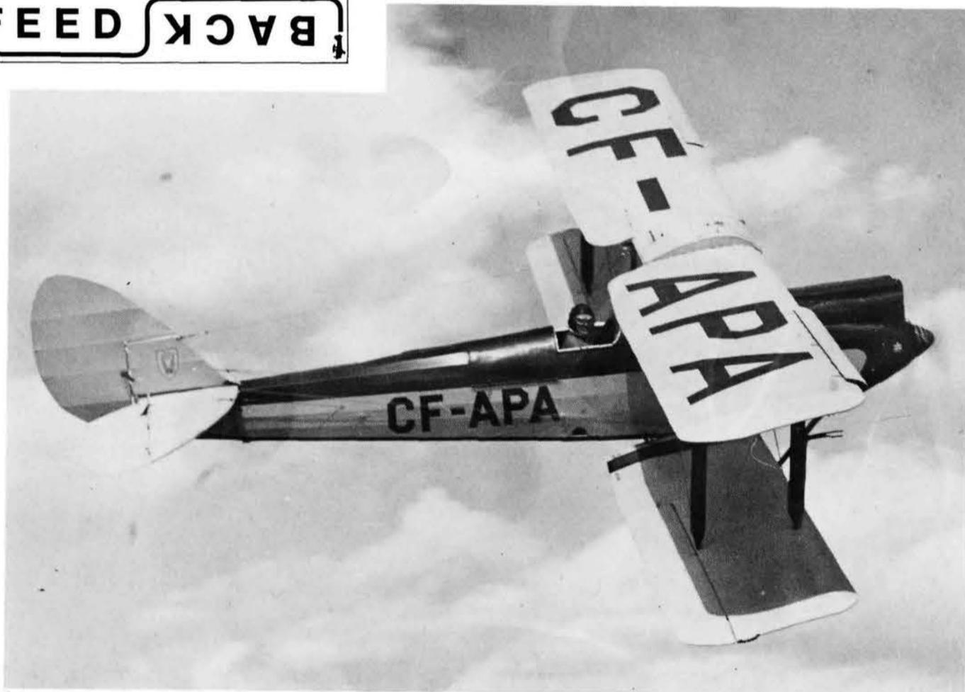
Right: A superb flying shot of c/n 1322 CF-APA after rebuild as a Gipsy Moth during the sixties. Features such as the fuel tank, trailing edge cut-out and leading edge slots can all be seen clearly from this angle.
