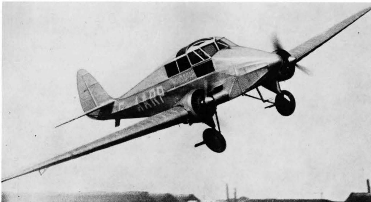
Left: G-AARP, two 45 hp Salmson 9-cyl radials, was the very first Monospar and was built by Gloster Aircraft. Originally called the SS1, later the ST-3, it is seen here in a flying demonstration in 1931. (Aeroplane via Jack Meaden)
