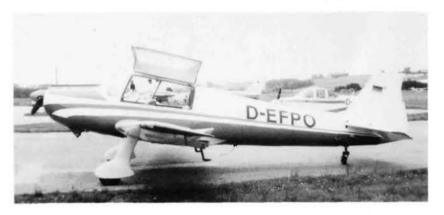
Above: D-EFPO c/n 262 at Eggenfelden on 5.7.81 (Peter Gerhardt) and below: HB-UXR c/n 264 at Zurich 5.7.64 (F.v. Bruggen via R.W.Simpson). Both illustrate the ease of access to all four seats of the BO 207 via the large upward opening doors.
