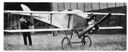
The third design, called the Piggott Military Biplane, (above) was the one we illustrated on p90/58. It was entered for the 1912 Military Trials at Larkhill as "29" but while being taxied by Parr it was damaged after hitting an obstruction and took no part in the Trials. It was underpowered with its 35hp Anzani 3-cyl radial engine and there is no record of it being flown successfully. It is believed that the Piggott machines were all disposed of in 1912.
