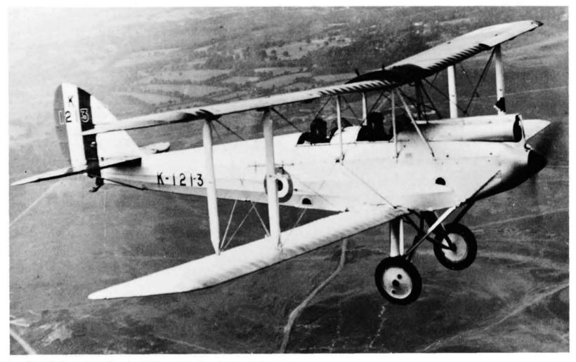
Above: DH.60M Moth K1213 c/n 1525, with fuselage stringers and upper leading-edge slots clearly visible, was delivered to the CFS in 1930 which is presumably when this manufacturer's photograph was taken. (BAe via Mike Hooks)
