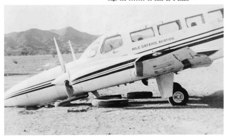
Right: Nile Safaris Cessna 404 Titan ST-AIT suffered a nosewheel collapse, presumably the incident at Gebeit in 1984 referred to in the register. (via P.Boswell)
