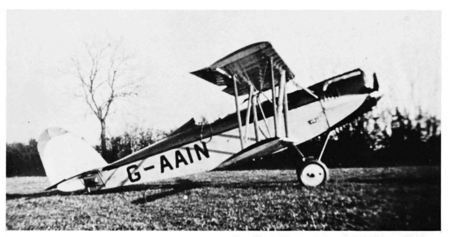
Above: Lord Apsley's Parnall Elf 2 G-AAIN, which differed from the Mk l (see page 90/11) in having the horn-balanced rudder, seen here in a field near Tetbury, Gloucestershire in the winter of 1938-9. (Jack Meaden)
