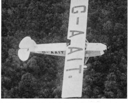
Above: Boulton & Paul P.41 Phoenix I G-AAIT parasol wing monoplane (40 hp ABC Scorpion flat twin) was of wood with fabric covering and was the only one built. Later it was modified to have a longer undercarriage with a wider track and was fitted with a 40 hp Salmson radial. (via J.Meaden)
