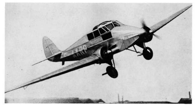
Left: G-AARP, two 45 hp Salmson 9-cyl radials, was the very first Monospar and was built by Gloster Aircraft. Originally called the SSI, later the ST-3, it is seen here in a flying demonstration in 1931. (Aeroplane via Jack Meaden)
