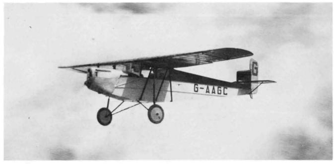
Left: G-AAGC was the second Koolhoven FK.41. It was brought to the UK to become the first Desoutter I, in which form the tailplane was lowered from the top of the fin to the top of the fuselage and changes were made to the cowlings to suit a 105 hp Hermes engine as seen here. (Jack Meaden)
