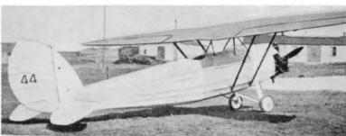
Top: The Clarke Cheetah G-AAJK c/n CC.1 (35hp Blackburne Thrush 3-cylinder radial) used a number of DH.53 parts and was designed as a convertible biplane/monoplane, the lower wing (from the Halton Mayfly G-EBOO) being removable. (JM) Above: The Clarke Cheetah G-AAJK again, this time as a monoplane in 1929 before obtaining a C of A. Purchased by four airmen of 600 Sqn in 9.30 it reverted to monoplane status and survived in this form until scrapped in 1937. (Aeroplane via Jack Meaden)
