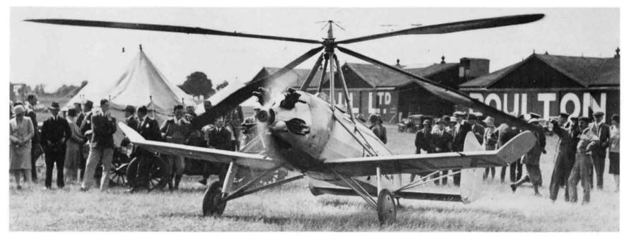
Above: G-AALA Cierva C.19 Mk II autogyro c/n 5135 (100 hp Genet Major) about to fly at the Norfolk & Norwich Aero Club Pageant at Mousehold aerodrome in 1930 piloted by A. H. Rawson. The C.19 was the first autogyro to be designed from scratch instead of using the fuselage of another aircraft. It also introduced the method of starting the rotor turning by tilting the tailplane so as to direct the slipstream upwards. (via Jack Meaden)
