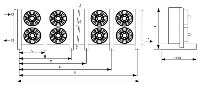
Unit shown has 2 fan lines - no. of motors between the feet is not contractually binding
