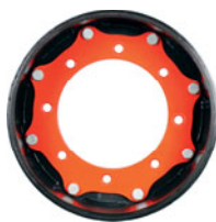
Hub Adapter MSPN 47462 CAI 481115 12 mm thick 1015 carbon steel / reversible 9.0" (228.6 mm) center dia. 8 x 10.75" bolt pattern 0.67" (17 mm) bolt holes, tapered Fits some Bobcat machines
