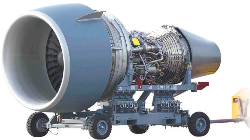
Shipping Stand for F138 Engines (used on Lockheed C-5M Super Galaxy Aircraft)
