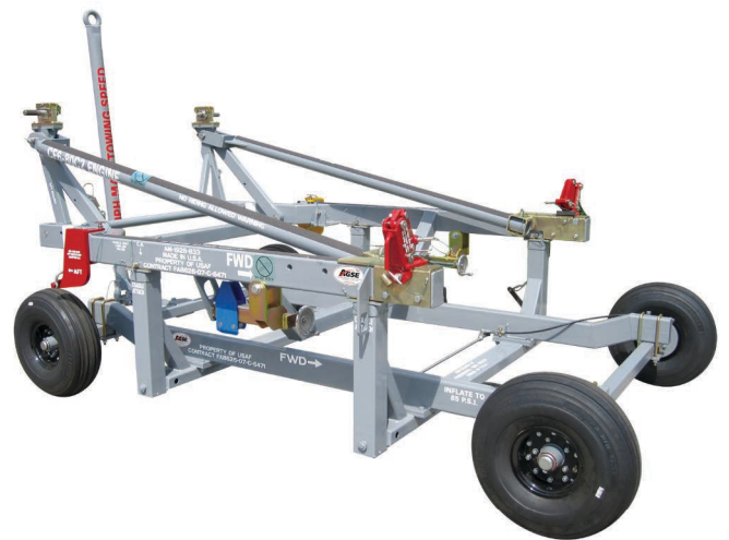
Pneumatic Tire Dolly for F138 Engines (used on Lockheed Martin C-5M Super Galaxy Aircraft)
