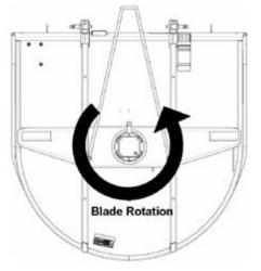
HX6 blade rotation **Single-spindle configuration** The HX6 Rotary Cutter features a single-spindle configuration.
