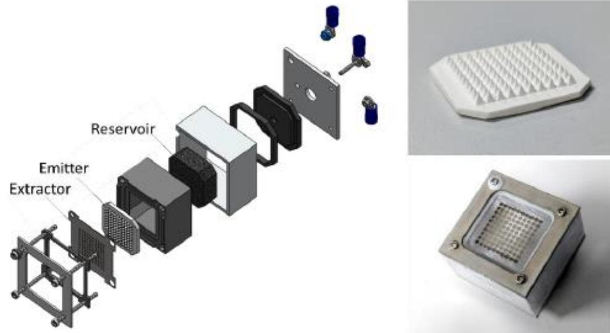
Figure 1. PET-100-MK2 thruster design and manufactured results.
