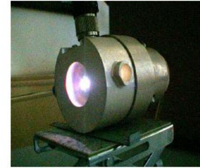
Fig.10 The picture of 1,000W MPT testing
