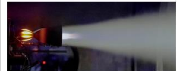
Figure 5: Steady-State Operation of HyNOx-22 in Vacuum Chamber
