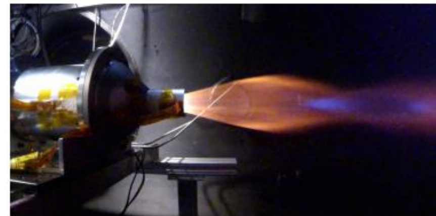
Vacuum chamber set-up with hybrid motor installed and torch igniter (left) and laser igniter (right)
