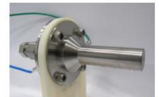
Figure 5. Picture of Rafael's R-800 Heaterless Cathode (ARC-2A)
