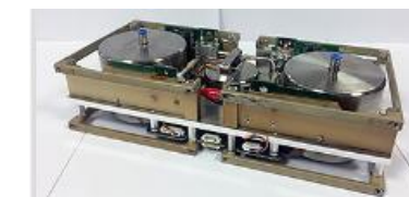
GomX-4B's cold-gas thruster system takes up two half-cubesat units at one side of the nanosatellite, with two spherical titanium tanks filled with liquid butane. It has four 1 mN thrusters, typically to be fired in pairs while keeping one set in reserve. Photo is courtesy of Nanospace.
