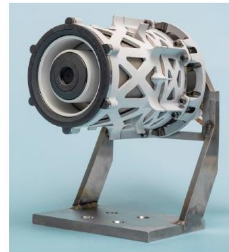
MaSMi-EM SN001 Hall thruster fabricated, assembled, and delivered by Apollo Fusion.
