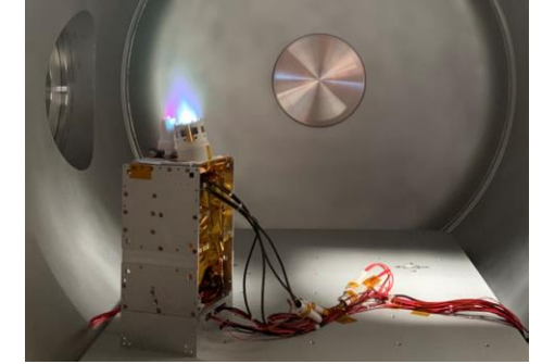
ExoMG™ – nano L during a coupling test [1]
