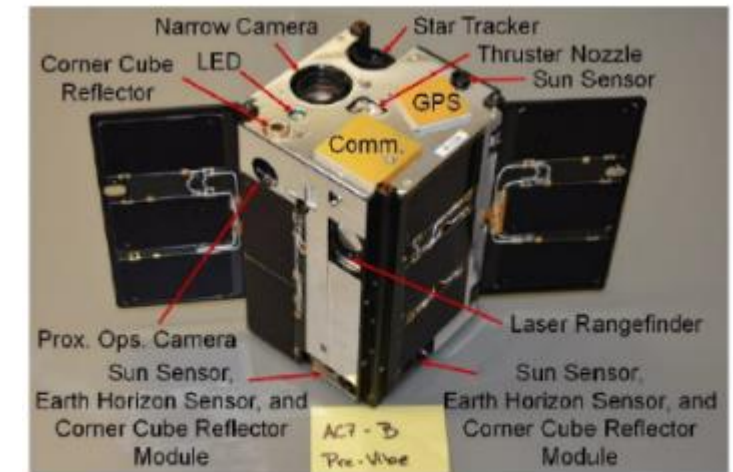
Figure 1: AeroCube-OCSD-B with deployed solar panels.
