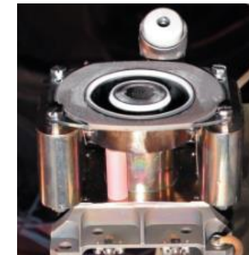
PlaS-40 thruster after 200 hrs operation time
