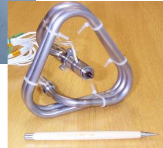
SNAP-1 vehicle, with butane propulsion system
