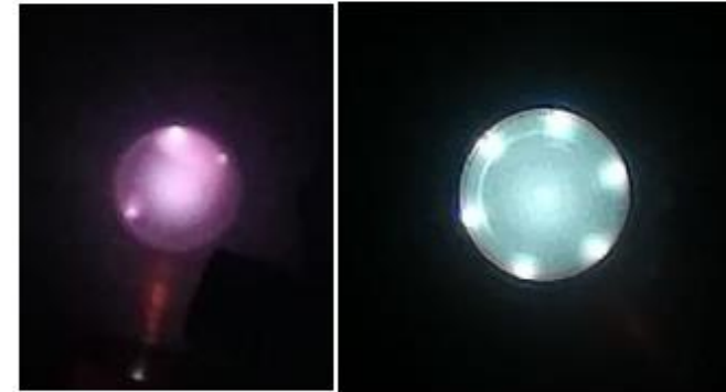
Fig. 3 Injector during ignition (left) and operation (right)
