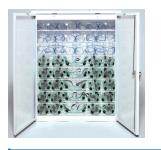
For sanitizing and storage of safety glasses or goggles. Holds 48 glasses or 40 goggles. Cycle controlled by timer. Pilot light confirms UV lamp in use. Shuts off automatically if double doors are open. Doors interlocked with tamper-resistant latches. Wall- or shelf-mountable with 7' grounded electrical cord. 24-gauge white enameled lockable steel cabinet. Germicidal lamp. No assembly required. Goggles/Glasses not included. Dimensions: 24 1/2"W x 32"H x 9 1/2"D.
