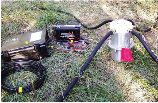
Fig. 7. Close up of infrasound sensor connected to four porous hoses. The porous hoses act as a windscreen for the sensor and are connected to a central manifold (the white segment) at the top of the sensor.
