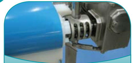
Grooved Spindle Guard for Increased Sanitation Access
