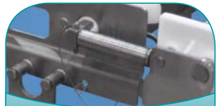
Stainless Steel Pin Tethers to Aid in Sanitation
