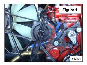
New parts are supplied as a Bearing Kit, #11496230 and a Pulley Kit, #11514152. This Service Bulletin gives step-by-step bearing installation instructions. Both kits will fit earlier units prior to the unit numbers listed above.
