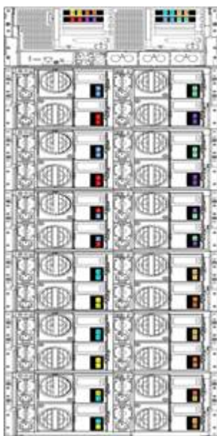
Apollo 4520 with 3xD6020 cabling diagram
