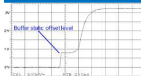
"Signature" Rising Edge Waveform
