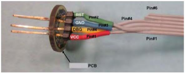
Figure 13. 6-Circuit Cable Modified for Programming
