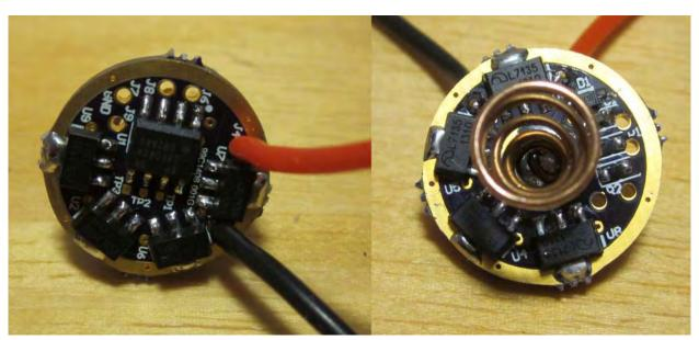
Figure 1. The LED Flashlight Driver Controller
