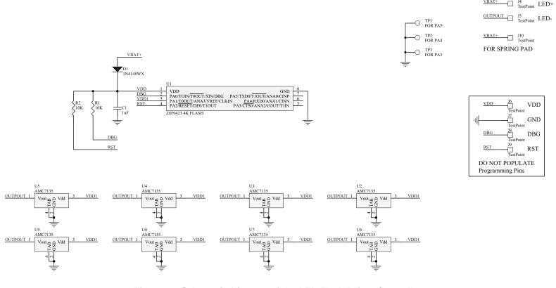
Figure 17. Schematic Diagram of the LED Flash Driver Controller
