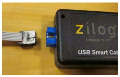
Figure 6. USB SmartCable Module and 6-Circuit Cable
