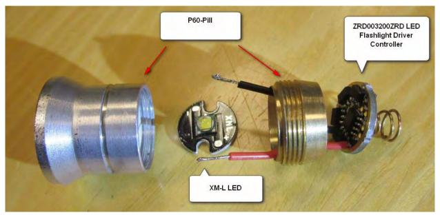
Figure 2. P60 Pill, LED, and LED Flashlight Driver Controller
