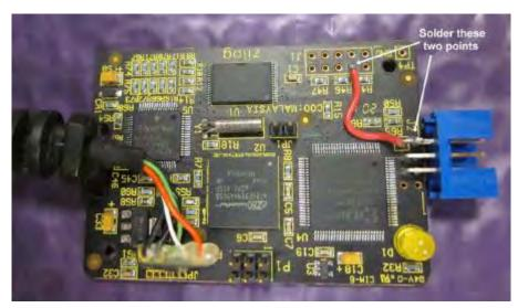
Figure 12. Solder Connections for Modifying the USB SmartCable
