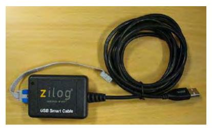
Figure 11. Programming Cable Shown with USB SmartCable Attached
