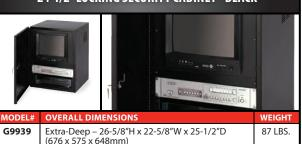
Cabinet sits on desk or wall mount, front door is 1-1/4" deep for electronic clearance and symmetrical for left- or right-hand mounting. 19" depth from front rack rail to inside back. NEMA electrical knockouts.
