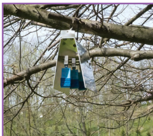
Outdoor sampling shelter protects multiple samplers.
