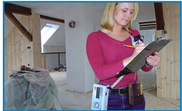
Attach to a pump to monitor dust levels in real time while collecting a gravimetric sample. SKC recommends using the AirChek 52/Sidekick pump. See pages 12-13.
