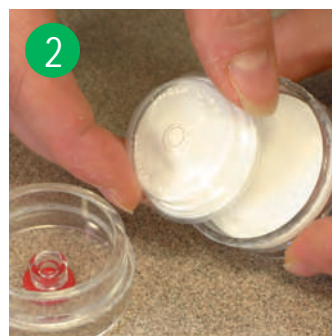
2 Weigh Accu-CAP and insert in cassette.
