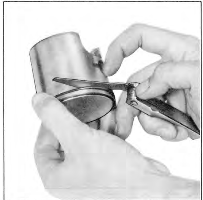
TOP RING/GROOVE CLEARANCE
