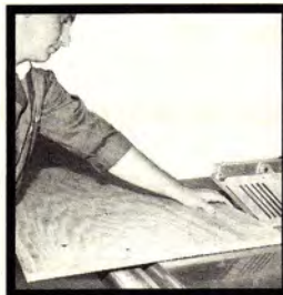
Extra Cut-Off Capacity table in front of blade is full 21" (533.40 mm) at 1" (25.40 mm) cut.
