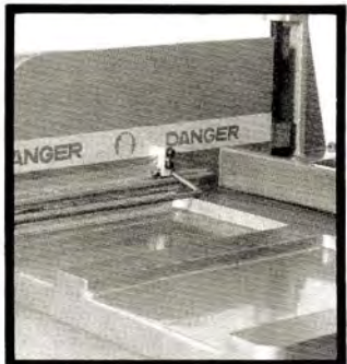
Recessed surface on top casting makes it easy to position stock for cutting.
