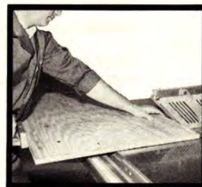
Miter Cut Accuracy - miter gauge adjusts easily, extends beyond table for wide stock.
