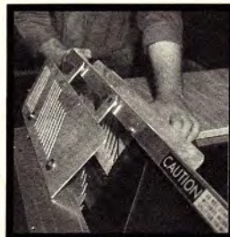
Individual Action of each guard leaf covers blade through entire tilt range. Saw blade is not exposed to operator.
