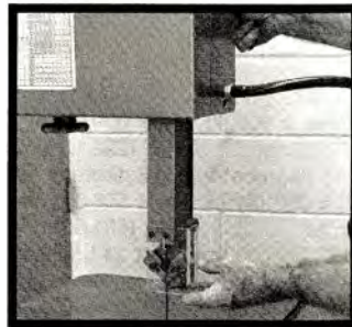
Counter-balanced guide bar makes guide and blade adjustment safe and simple. Note telescoping guard enclosing blade above guide.
