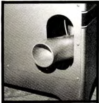
Built-in dust collection chute is an integral part of the design.
