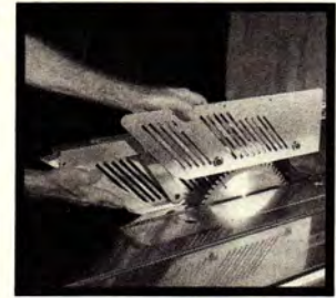
Guard hold down - a unique spring loaded hold down helps prevent panel lift by the blade during scoring operations.
