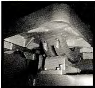
Heavy Duty 6" (152.40 mm) single-action trunnion for maximum rigidity. Adjust table 45 degrees right, 15 degrees left.
