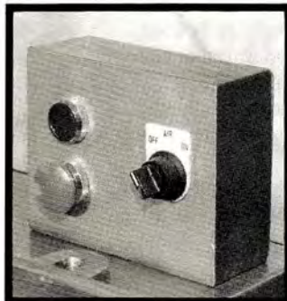
The on/off and air control switches are located on the top/rear of the machine for easy reach.
