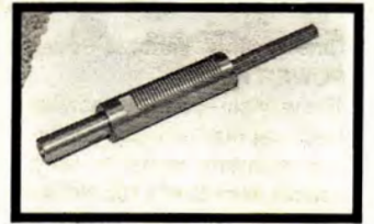
6 Spine Spindle of carbon steel is mounted in four heavy-duty sealed ball bearings to absorb both radial and vertical thrust. Standard spindle taper is #3 Morse.
