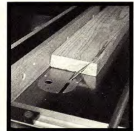
ADDED SAFETY—blade tilts away from fence to guard against possible binding of material against fence. Shown without guard for illustration only.
