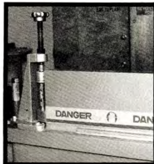
Guard/clamp height is easily set using the adjusting knob.
