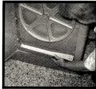
Convenient, removable chip pan is located just below lower wheel.
