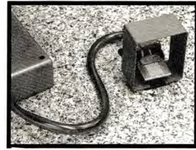
Pneumatic quill is controlled by pneumatic foot pedal. May be used for drilling or locked for routing.
