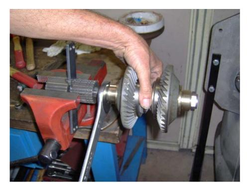
Insert and tighten the fixing nut (ref. n°9)
