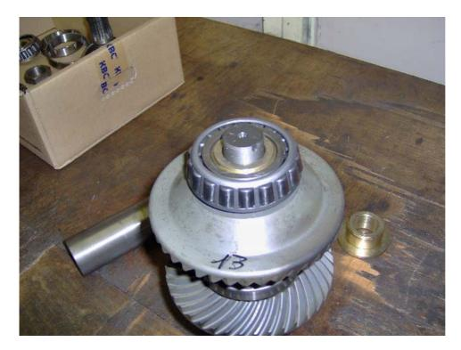
Remove the fixing nuts (ref. n° 9) Warm the bearings (ref. n° 10) up to 120 °C, put them on the bearing housing (ref. n° 8)
