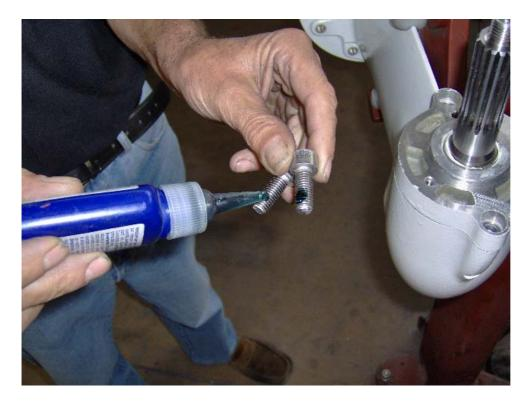
Position the support all the way down. Put in the fixing screws ( rif. n° 83) applying a drop of thread locker Tighten and fit the helicoil ( rif. n° 90)
