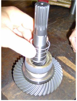
Put the clutch body (ref.  $n^{\circ}2$ ) into the sahft (ref.  $n^{\circ}1$ ), make sure it has enough play to the spline and it moves freely. Put on the opposition spring (ref.  $n^{\circ}12$ )
