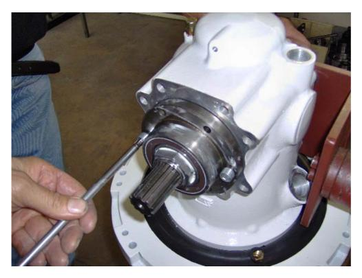
Put the gear group into the cover group, tighten the fixing screws, Put on the oil seal (ref  $n^{\circ}$  18)
