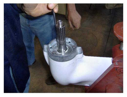
Assemble the zinc ( rif.  $n^{\circ}$  84) and tighten with screws ( rif.  $n^{\circ}$  91)
