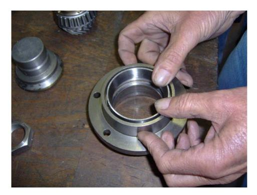
Put the bearing bowl (ref. 19 and 22) into the bearing housing (ref.  $n^{\circ}$  14) all the way down.
