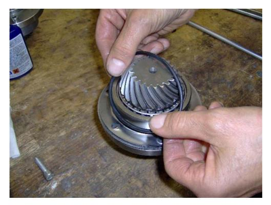
Put on as shims as to add 0.05 mm to the value detected by the thickness gauge. Put the o-ring (ref.  $n^{\circ}16$ ) in its location, add grease if necessary.
