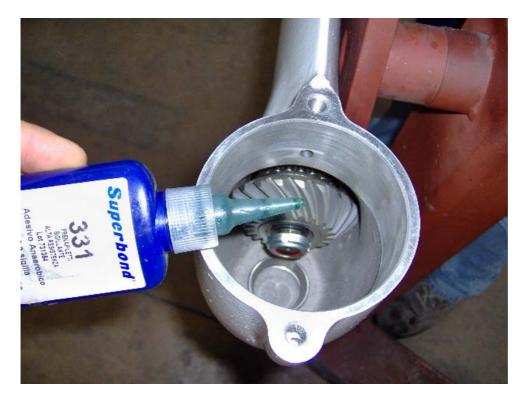
Disassemble the adjustment tooling, position the shims, reassemble the components as shown previously, when reassembling the nut (rif.  $n^{\circ}$  70) use drops of thread locker.
