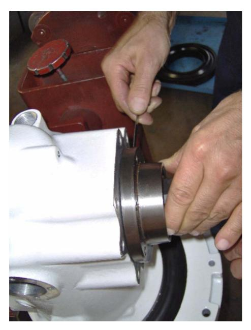
Put the gear group into the cover group, verify the left distance between the gear group and the case
