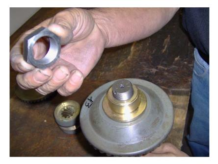
Put on the bearing housing (ref. n°8), screw the lock nut (ref. n° 9)
