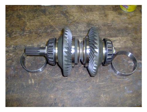
Position the preassembled clutch group with the thrust blocks of the respective bearings
