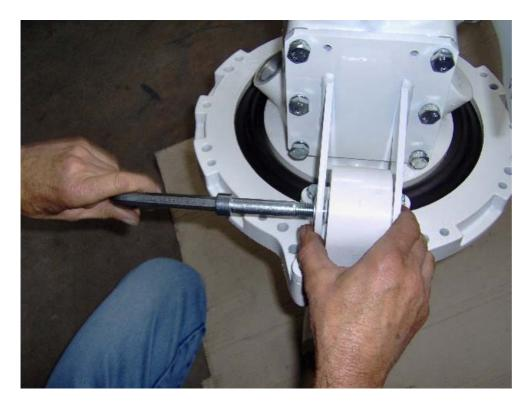
Apply support ( rif. n° 95) and tighten with bolts ( rif. n° 101) Apply antivibrating bracket ( rif. n° 96 ) and fixing screw ( rif. n° 98), tightening it
