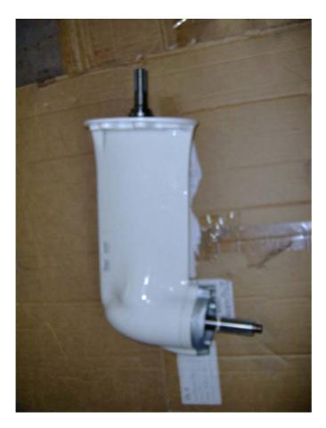
Manually check the shaft spin and the play between the tapered pairs. There should be no crawling during the spinning
