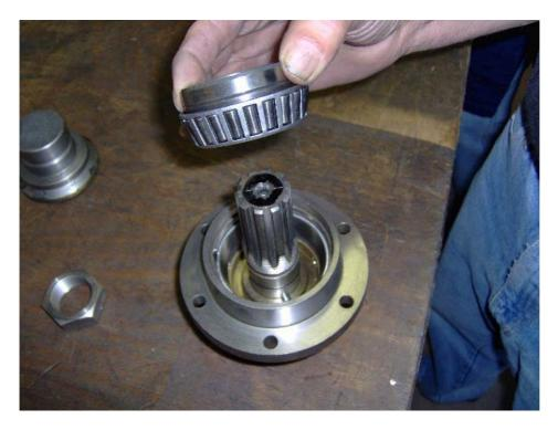
Put on the previously assembled shaft internally to the bearing housing. Put bearing (ref. n°22) onto the bearing housing (ref. n° 23) Put the bearing all the way down into the shaft
