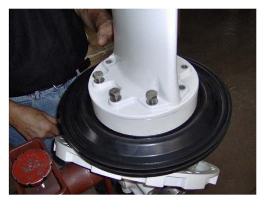
Insert the retaining ring ( rif.  $n^{\circ}$  50) Join the upper part with the lowe part of the gearbox, place the fixing screws ( rif.  $n^{\circ}$  72) and tighten
