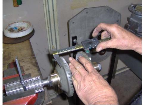
Measure the height of the clutch group, the value must be 83.02 mm. If it is not, increase or decrease the thickness by adding or removing some shims (ref. n° 3)
