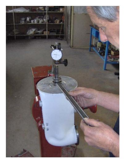
On the end of the shaft, assemble a dial gauge and detect the axial shifting as per scheme  $n^{\circ}3$ .
