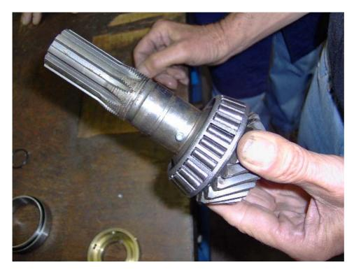
Warm up bearing (ref.  $n^{\circ}19$ ) up to 120 °C Put it as per picture all the way down into the shaft (ref  $n^{\circ}$  17) Insert the drag pin of the oil pump (ref.  $n^{\circ}$  20)
