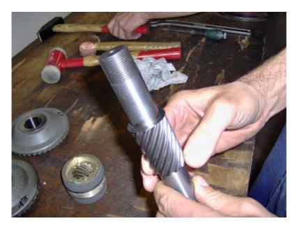
Put shim (ref.  $n^{\circ}3$ ) into the shaft (ref.  $n^{\circ}1$ ) until it hits the splined part of the shaft.
