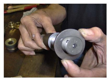
Put shim (ref.  $n^{\circ}4$ ) all the way down into the shaft.
