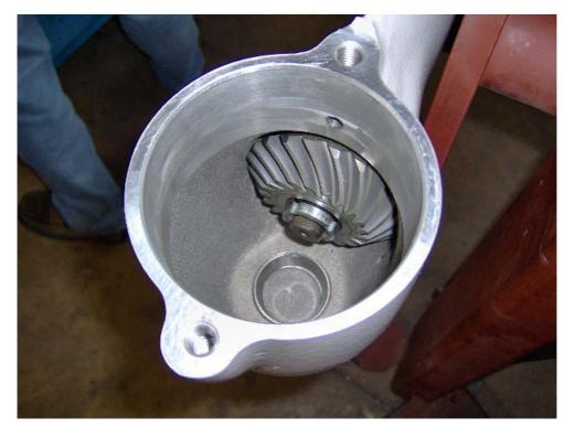
Detect gear (ref. n° 68) measurement as per scheme n° 3. Put the bearing (ref. n° 66) on the gear, insert transmission shaft (rif. n° 60), assemble the gear and screw the lock nut (rif. n° 70)
