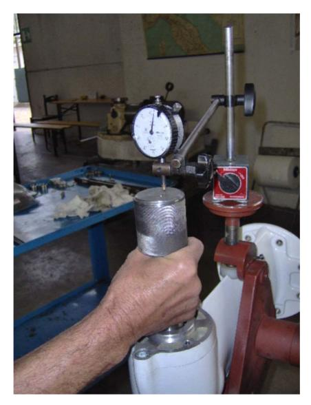
Put the bearing bowl (ref.  $n^{\circ}$  19) into the bearing housing (ref.  $n^{\circ}$  78). Insert the support and use the bolts to fix it.
