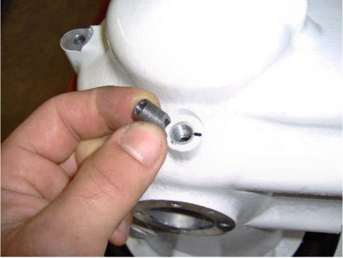
Put the fitting on the location of the breather plug, screw the fitting all the way, positioning the chamfered part as per the photo. Screw the breather plug (rif. n° 53)
