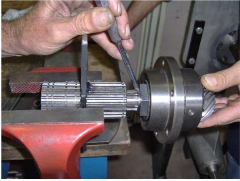
Insert and tighten the fixing nut (ref. n° 24) Rivet the thread using a pin to avoid its unscrewing, in two opposite locations
