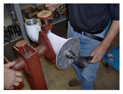
With the proper tool (tool SP60 -07), hold steady the shaft in order to prevent its spin, screw lock nut (rif. n° 70) and (rif. n° 61)
