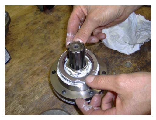
Put the oil seal (ref. n° 25) in its position, adding grease in its location to make the assembly easier.
