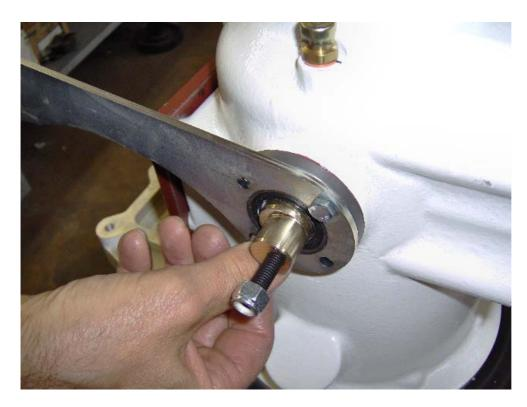
Put in the fixing screws (ref.  $n^{\circ}$  88) with thread locker, and tighten. Put on the drive bracket (ref.  $n^{\circ}$  38), tighten the fixing screws. Out the bushing for the breather plug into the threaded hole. Screw the breather plug (ref.  $n^{\circ}$  53 e 54).
