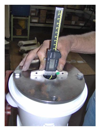
Verify the measurement on the top of the shaft with a depth gauge. Disassemble tool SP 60-02, remove the gear group, remove the clutch group. Adjust the bearings, applying a 0,05 mm preload, dividing the shims into equel parts under the thrust blocks of the bearings (ref. n° 10)
