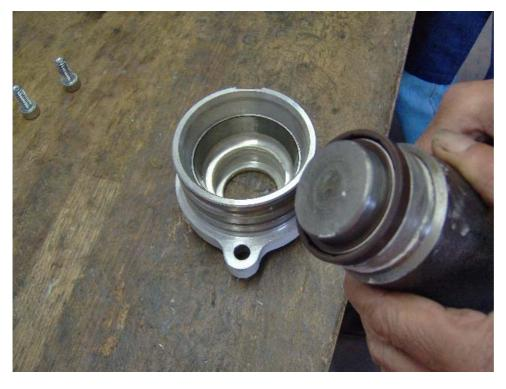
Put oil seals (ref. n° 79) in the support (ref. n° 78) as shown by the cross section drawing. Assemble the O-rings (rif. n° 80) and grease their surface to make their assembly easier.
