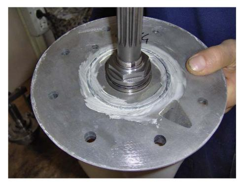
Put the o-ring (rif. n° 65) in its location, apply grease to make the assembly easier
