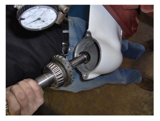
Put the bearing bowl (ref. n°82) into the lower cover group. Insert the output gear group, already preassembled.
