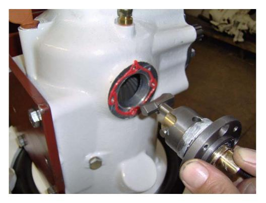
Apply layer of sealant paste as shown by the picture, insert the drive group previously assembled
