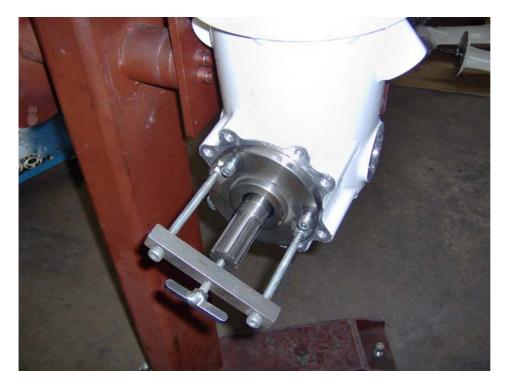
Inserit the gear group previously preassembled, apply tooling (tool SP 60-03) as per the picture, on the input shaft.
