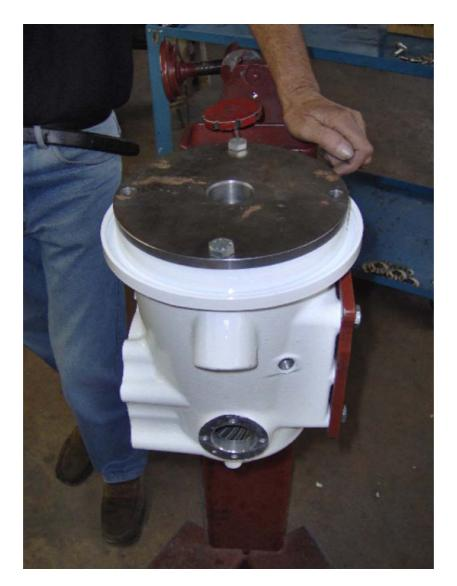
Insert the tooling (tool SP 60-02) to center the clutch group into the cover upper assy. Tighten it with the two screws.
