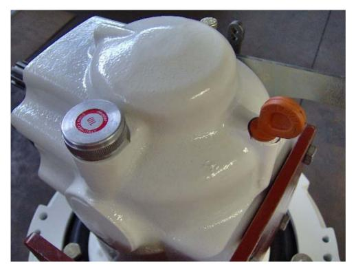
Finish the upper part of the gearbox, applying the oil dipstick and the oil filling plug. Apply and tighten the lock plug on the membrane( rif.  $n^{\circ}$  44)
