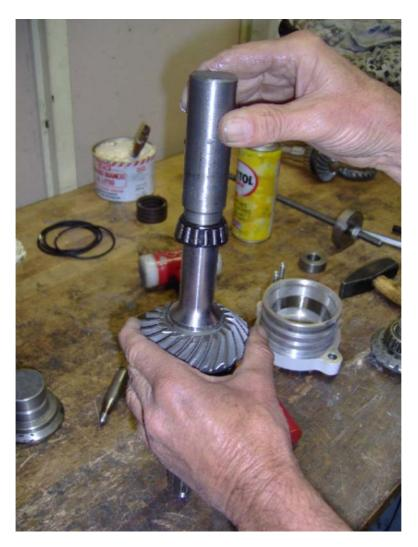
Put the gear (ref. n°74) on shaft (ref. n° 73). Insert bearing (ref. n° 82), with the help of a stopper if necessary (tool SP60-05)
