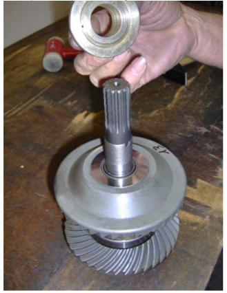
Warm up ring (ref. n°5) up to 120 °C, position it all the way down into the shaft. Insert the two cages (ref. n° 6) Put on the clutch gear (ref. n° 7) Position the bearing housing (ref. n°8)
