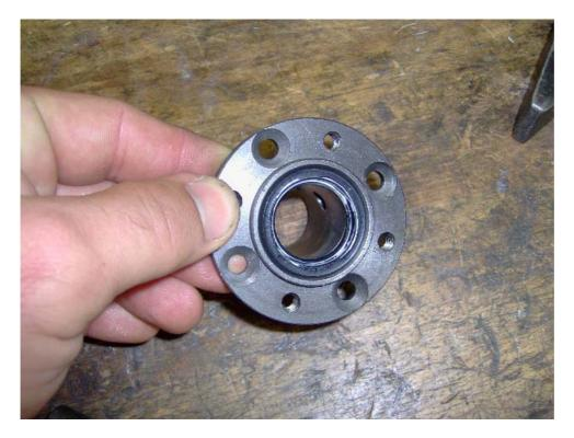
Put on the oil seal (ref. n° 29) internally to the support of the drive group (ref. n° 28) Grease the oil seal location to make easier the insertion, put it down using a stopper if necessary
