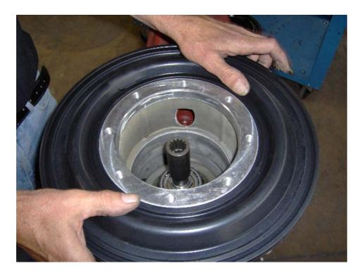
Insert the preassembled clutch group. Put the sleeve (ref. n° 63) into the shaft. Put in the two membranes ref. n.41 and later ref. n.42.
