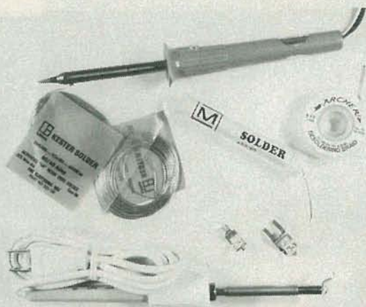
FIG. 1—SMC's CAN BE HAND SOLDERED using only the common tools and materials shown here.
