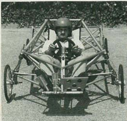
THE SOLAR-POWERED CAR's spaceframe and chassis gets its first test drive in California. Dr. Alec Brooks of AeroVironment, Inc., is checking its rigidity, handling and suspension. The lightweight spaceframe, made of aluminum tubing, will become a sleek, high-tech racer when covered by its integral body, canopy and solar panels.
