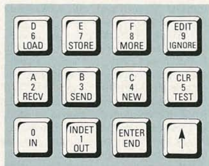
FIG. 5—LABEL THE KEYS as shown here for installation in a case. Otherwise, reverse labels from left to right.
