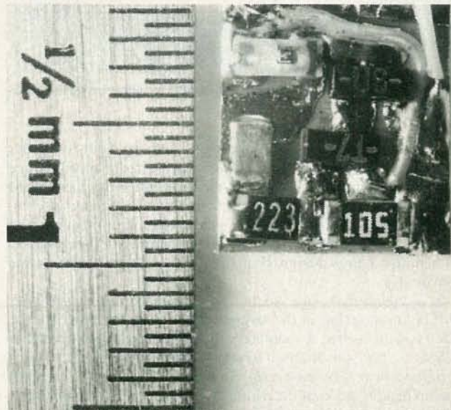
FIG. 1—MICROMINIATURE INFRARED LED transmitter assembled by the author.
