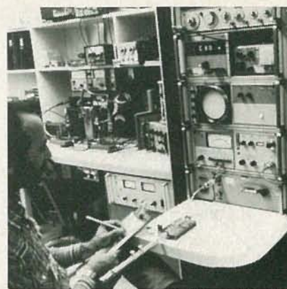
FIG. 7—RF POWER TRANSISTOR IMPEDANCES are determined by measuring the characteristics of a working circuit.
