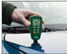
Measuring the thickness of automotive paint
