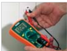
Displays AC Voltage of an outlet receptacle
