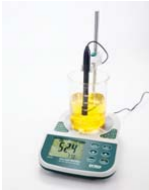
Magnetic stirrer with adjustable clamp for hands free testing
