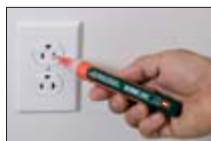
Non-contact Voltage Detection
