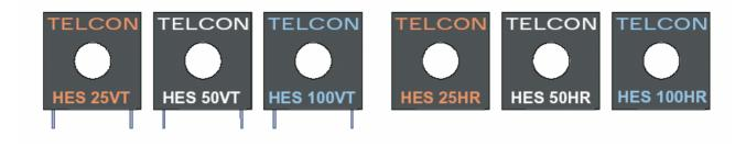
The HES series of Hall Element and coil assemblies enable the implementation of a full Hall Effect Current Transformer by the addition of the requisite electronic circuitry, suitable for measuring currents up to 100A. They are supplied as a free-standing component, enabling the user to configure a closed-loop Hall Effect current transformer to their own specification.
