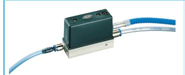
Air/electronic converters convert the signals from pneumatic measuring equipment (air pressure) into electrical signals. The piezo-electrical measuring system means that the **Millimar** X 1941 air / electronic converter can be finely aligned with most of the pneumatic systems on the market. The **Millimar** X 1941 has an analog signal output. It can therefore be very easily connected to the measuring computer and control system.
