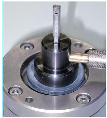
Jet air plug gage with floating bearing
