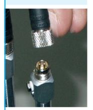
Cable and probe can be seperated with the plug-in connector.
