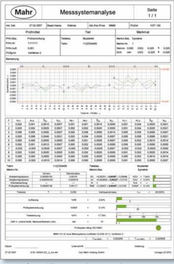
Record of a capability test according to Procedure 2
