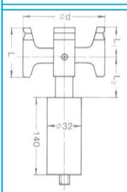
6001 Z hard-chrome plated, for indicator instruments (dia. 80 - 100 mm)
