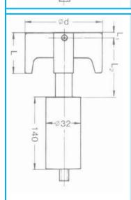
6011 Z hard-chrome plated, for indicator instruments (dia. 80 - 100 mm)
