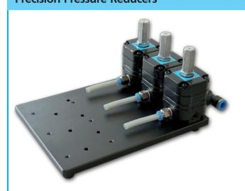
These devices create the normal pressure of 2 bar needed to operate the air/electronic converter from the overpressure of approx. 5 bar. Since this pressure must be precisely constant, the precision pressure reducers from Mahr are prescribed for the operation of the converter **Millimar** 1940.
