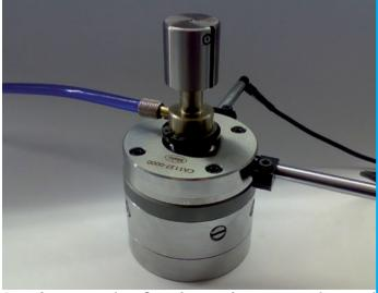
Jet air plug gage mounted on a floating bearing with position query to diameter and determination of position
