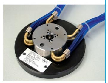
Taper jet air ring gage with 2 measuring paths on 2 planes each to test 4x diameter, 2x taper angle, 2x taper pitch
