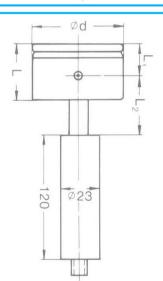
6001 Z hard-chrome plated for indicator instruments (dia. 5 - 80 mm)
