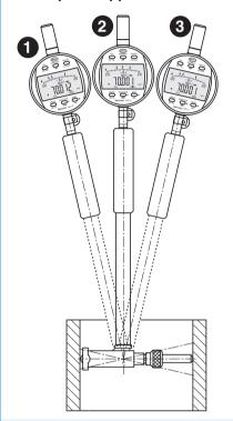
With a 2 point inside measuring instrument the point of reversal is automatically determined through rocking back and forth. The actual value is detected and stored by the MIN function and indicated in the display (3).
