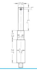
6012 Z hardened, for indicator instruments (dia. 3 - 5 mm)
