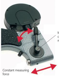
Measuring spindle has a lever controlled retraction and is mounted in a long guide way
