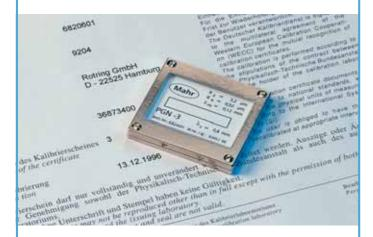
Surface roughness standard with a sinusoidal groove profile. Profile depth approx. 3 µm (120 µin), groove spacing approx. 0.12 mm (.00472 in). For checking the roughness measuring station. The following types are available:
