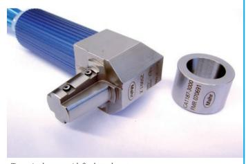
Taper air plug gage with fixed attachment
