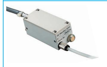
Air-controlled probes are becoming more and more widespread in dimensional metrology. Air / electronic converters convert the measuring signal (air pressure) into an electronic signal. Millimar 1940 is particularly well-suited to measurements with narrow tolerances. Its cutting-edge carrier frequency measuring system means it can be connected to the evaluation instruments in the same way as an inductive probe.
