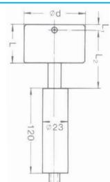
**6011 Z** hard-chrome plated, for indicator instruments (dia. 5 - 80 mm)
