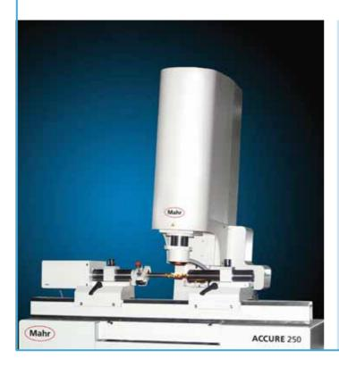
Precision measurements of helical cutting tools thanks to setting the pivoted measuring head to the lead angle.
