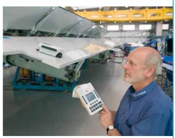
Roughness measurement on wings (Airbus)
