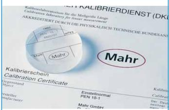
Depth setting standard for the static calibration of the vertical stroke of all skidless, single-skid and dual-skid probes. Groove depth. approx. 10  $\mu$ m,  $\varnothing$  44 mm.
