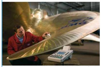
Roughness measurement on ship propellers (Mecklenburger Metallguss)
