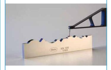
The contour standard KN 100 was developed in cooperation with the PTB. Testing for confirmation and acceptance purposes can now be conducted traceable back to the PTB due to concrete reference to realistic geometries.
