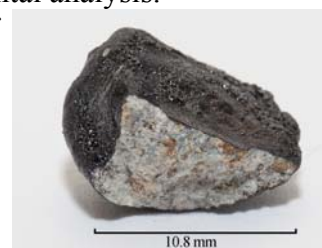
Fig. 1. Photographs of two fragments of “Chelyabinsk” meteorite studied. (left) a fragment covered with a black flow crust; (right) a fragment with a freshly cleaved grey surface
