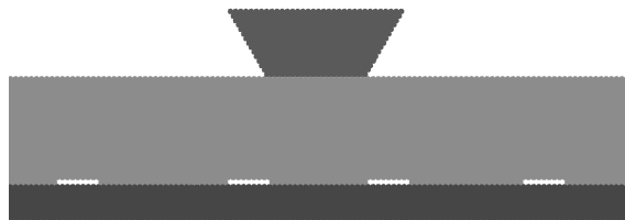
Figure 2: Fragment of simulated system with defect structure at the interface coating/substrate (length of cracks is equal to 24 nm)
