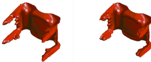
Figure 1: Unstable displacement front pattern shown by surface s(x, y, z) = 0.25 in space. Left plot corresponds to the fine mesh 100 \times 100 \times 50 , right to the coarse one 80 \times 80 \times 40 . Time moment is t = 0.129
