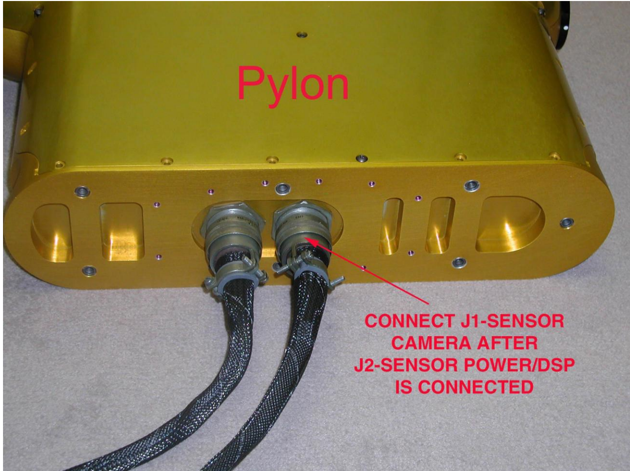
Figure 2.2.9: Connecting the sensor camera cable to the Sensor Head.
