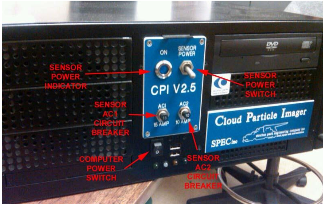
Figure 2.2.1: Front of the Data Acquisition System
