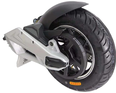
10inch 90 1KW IPM Motor Kits
