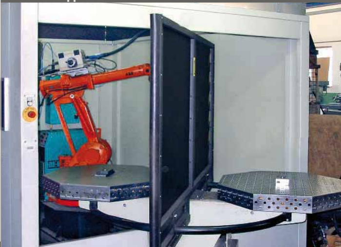
Two 3D welding tables Okto in alternating operation in robot cell. For optimum robot use: possible through prefitting.
