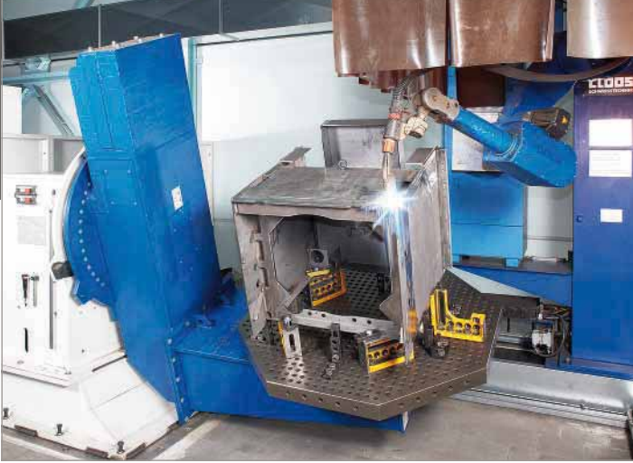
3D welding table Okto and accessories, on L positioner
