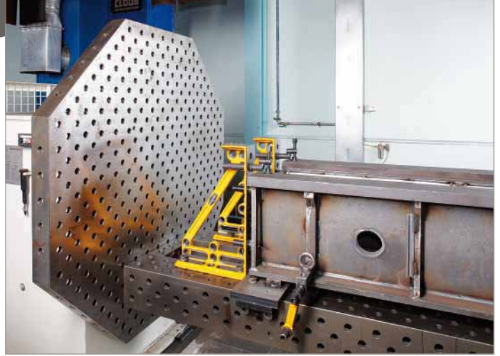
3D frame made up of Demmeler system components: spacer angle U-shape and two 3D welding tables Okto on rotary manipulator with counter bearing
