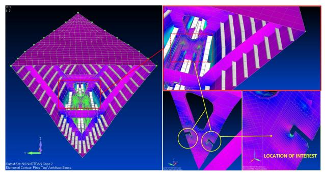
Figure 4-14: Local Model in the Critical Region of Side Shell & Bottom Web Frame (Bow Section)
