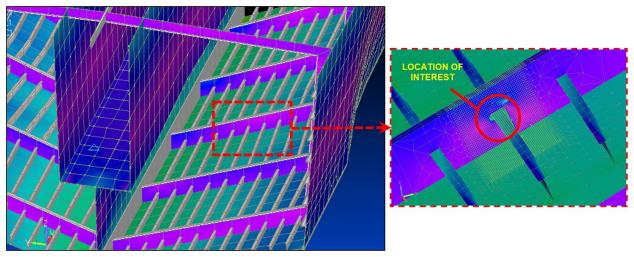
Figure 4-15: Local Model in the Critical Region of Bottom Web Frame (Midship Section)
