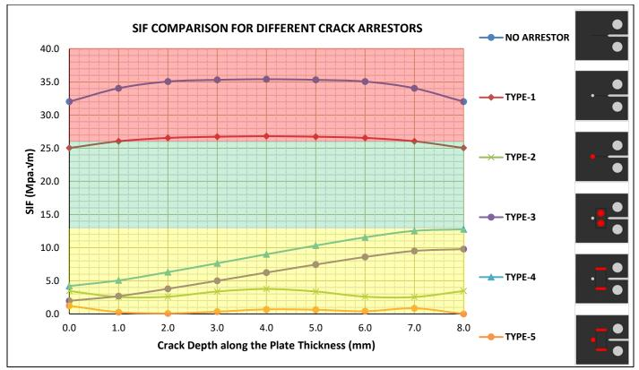
Figure 5-10: SIF Comparison for Different Crack Arrestor Types
