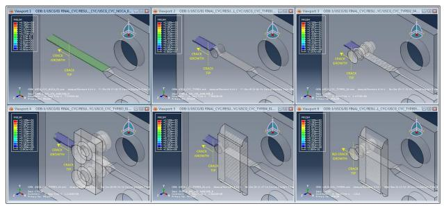
Figure 5-11: Performance under Cyclic Loading for Different Arrestors
