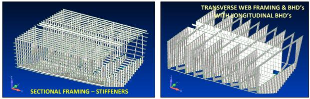
Figure 4-10: Global Model for the Midship Section
