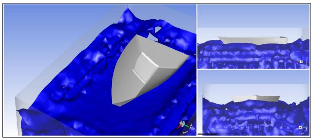
Figure 4-6: CFD Analysis – Representing Fluid Contact with the Vessel.
