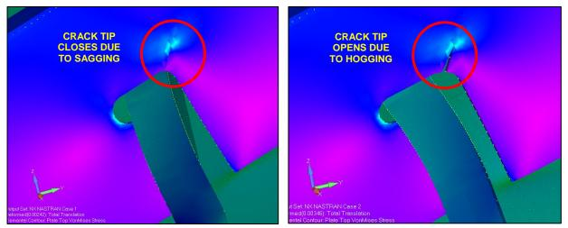
Figure 4-16: Crack Tip Behavior during the Sagging and Hogging Bending Moments
