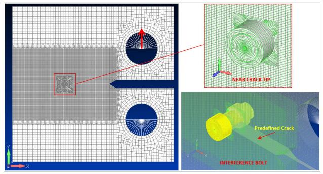
Figure 5-4: CRACK ARRESTOR TYPE-2 - CAH (Crack Arrest Hole) with Interference Bolt
