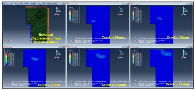
Figure 4-20: Von Mises Stress Contour for Progressively Increasing Crack Lengths – Midship Section
