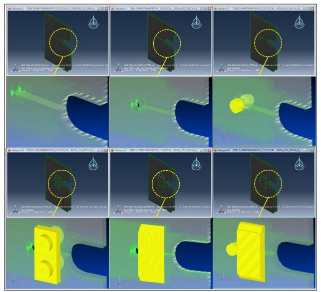
Figure 6-5: Introduction of different Crack Arrestors – Bow Section
