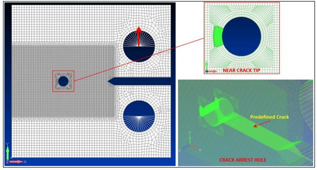
Figure 5-3: CRACK ARRESTOR TYPE-1 - CAH (Crack Arrest Hole)
