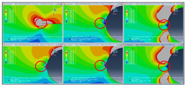
Figure 6-7: Von Mises Stress Contour Focused at the Crack Tip Region – Bow Section
