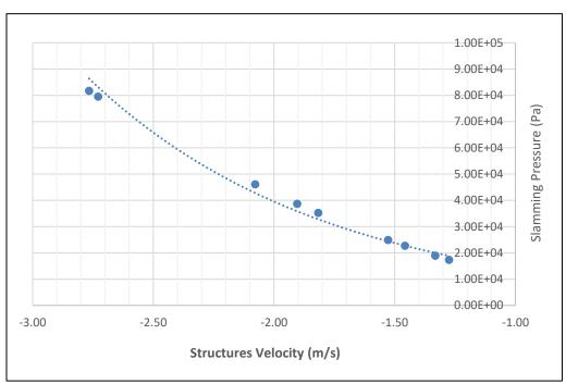
Figure 4-9: Slamming Pressure Estimate for Different Loading Conditions
