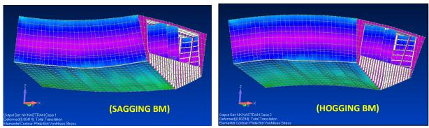
Figure 4-11: Vessel Stress Contours & Deformation due to Bending Moments
