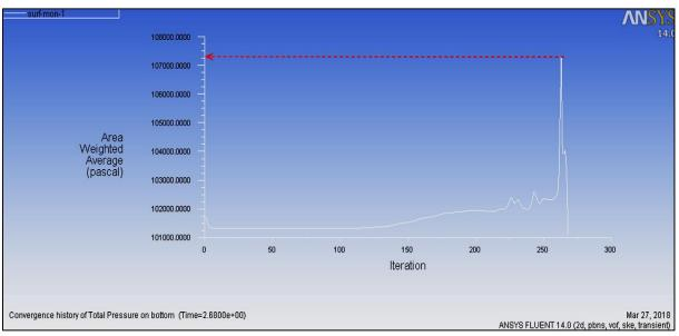
Figure 4-7: Plot for Average Slamming Pressure per unit Area over Time
