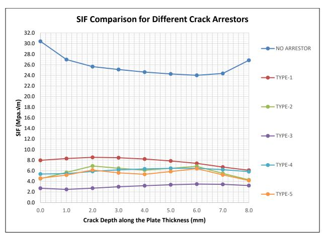
Figure 6-8 below compares the SIF's for different crack arrestor types at the critical bow section, which infers the reduction in stress intensity factors after introduction of the crack arrestors.
