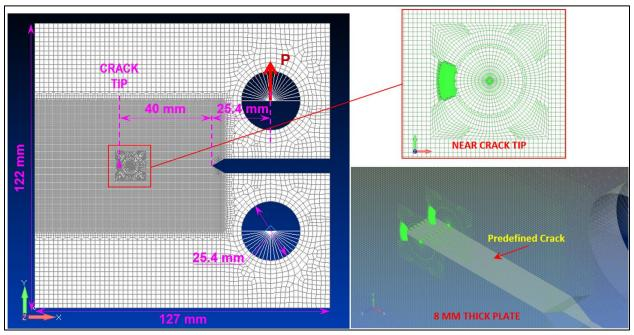
Figure 5-2: Base Specimen without a Crack Arrestor
