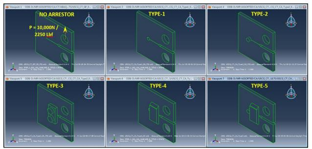
Figure 5-1: Different Crack Arrestors Considered for Study
