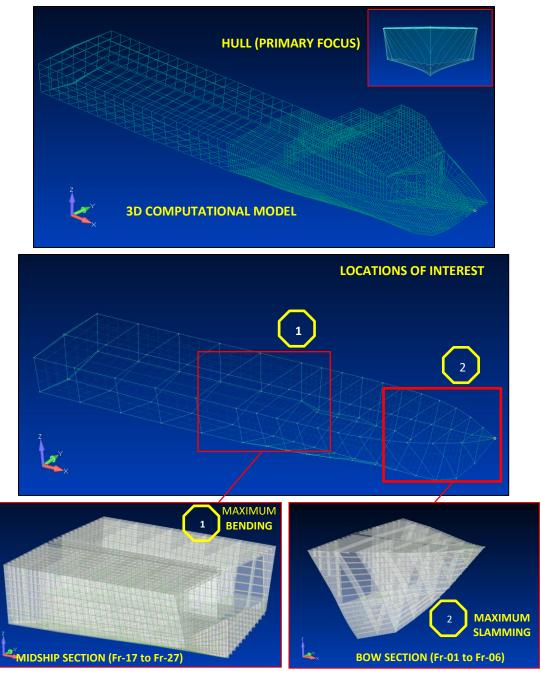
Figure 4-2: Development of 3D Analytical Models
