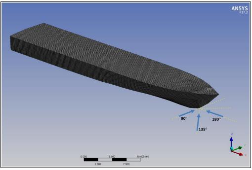
Figure 4-3: Hydrodynamic Analysis – Irregular Waves
