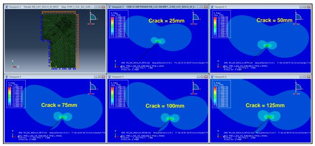
Figure 4-21: Von Mises Stress Contour for Different Crack Lengths (focused at crack tip region) -Midship Section
