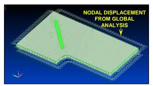
Figure 4-18: Conversion from Plate to Solid Elements and Application of Nodal displacements
