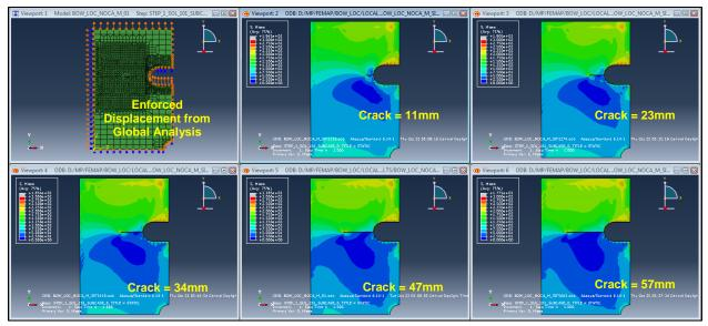
Figure 4-24: Von Mises Stress Contour for Progressively Increasing Crack Lengths – Bow Section
