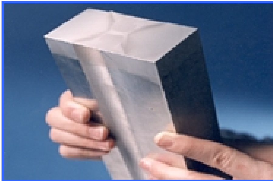
Figure 40 Double Sided Friction Stir Weld in 75 mm Thick Aluminum Extrusion
