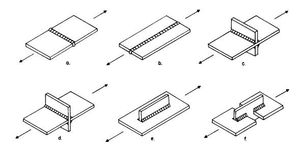
Figure 3-1 Typical Small Specimen Geometry
