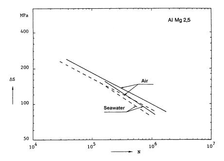
Figure E-9; Transversely welded plate with V- connection; Alloy AIMg2.5; R = 0.1;
