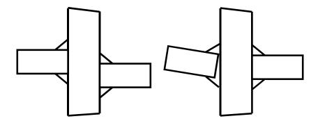
Figure 4-9 Typical Misalignment Problems During Fabrication
