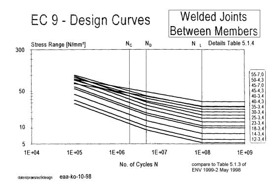
Fig. 5.2.4\* Design Curves  $\Delta \sigma$ -N for welded joints between members
