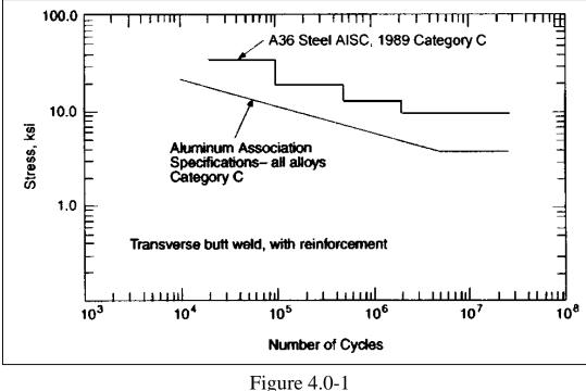
Figure 4.0-1 FATIGUE DESIGN CURVES FOR ALUMINUM AND STEEL
