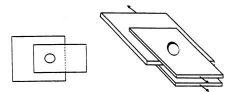
8.1(A) — RIVETED OR NON-FRICTION BOLTED JOINT — NET SECTION STRESS (AXIAL LOAD)
