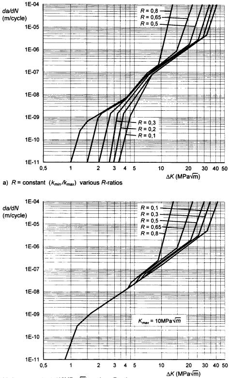
b)  $k_{max} = \text{constant} (10 \text{MPa}\sqrt{m}) \text{ various } R\text{-ratios}$
