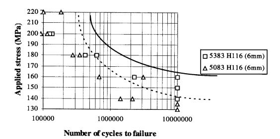
Figure 3-21 Fatigue Tests on 5083 and 5383 conducted at laboratory
