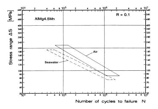
Figure E-1; Transversely welded plate; Alloy AlMg4.5Mn; R = 0.1;
