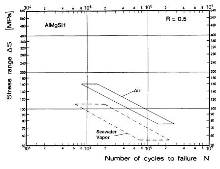
Figure E-12; T-Joint connection; Alloy AlMgSi1; R = 0.5;
