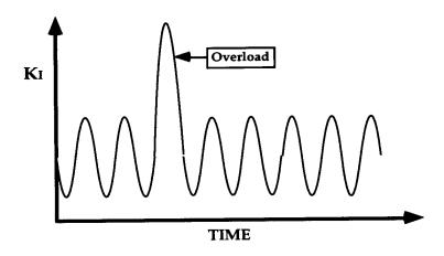
Figure 6-5 Peak Overload in Constant Amplitude Field
