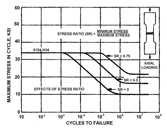
Figure 3-7 Effects of Stress Ratio on 5154-H34 Aluminum
