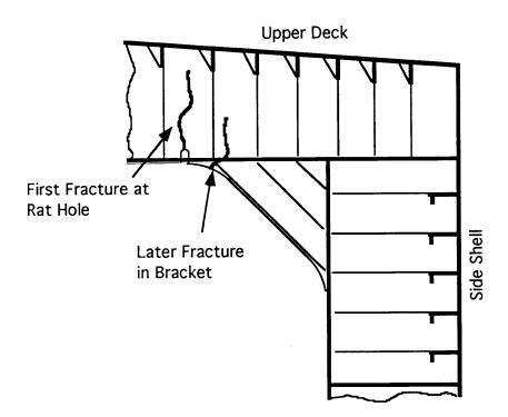
Figure 3-11 Typical Crack Initiation Sites
