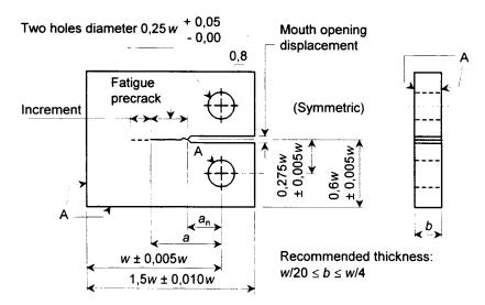
Fig.B.3.1. Typical crack growth specimen (example from ref.B.8.3)
