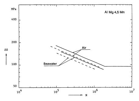
Figure E-13; Cruciform Joint; Alloy AlMg4.5Mn; R = 0.1;
