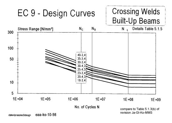
Fig. 5.2.5\* Design Curves  $\Delta \sigma$ -N for crossing welds and built-up beams
