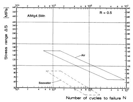
Figure E-11; T-Joint connection; Alloy AlMg4.5Mn; R = 0.5;
