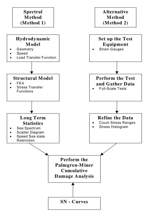
Figure 2-1 Flow Chart For Load Prediction
