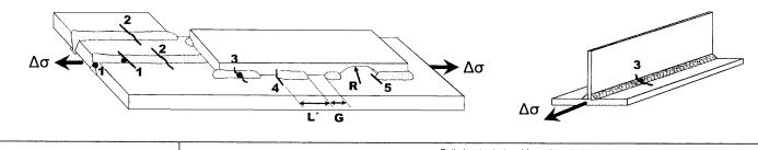
Table 5.1.3\* Detail Categories for Members with Welded Attachments - Longitudinal Welds
