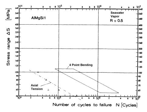
Figure E-2; Transversely welded plate subjected to both axial tension and 4 point bending; Alloy AlMgSi1; R-ratio = 0.5;
