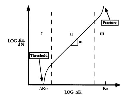
Figure 3-14 Typical Fatigue Crack Growth Rate, FCGR Curve
