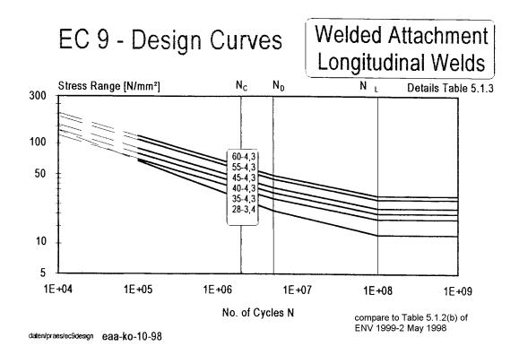
Fig. 5.2.3\* Design Curves  $\Delta \sigma$ -N for members with welded attachments / longitudinal welds
