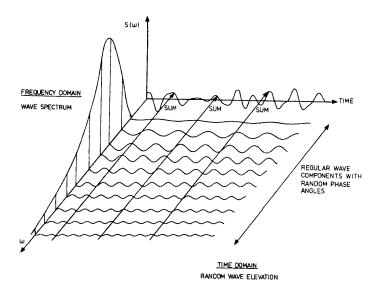
Figure 2-4. A schematic description of a sea spectrum.
