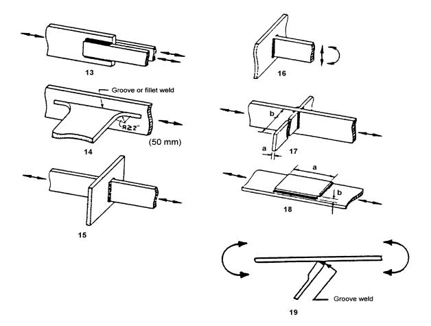
Figure 4–10 Typical Construction Details (Cont'd)
