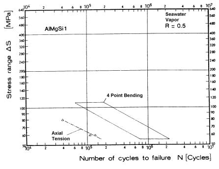
Figure E-16; T- Joint; Alloy AlMgSi1; R = 0.5;
