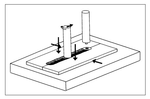
Figure 3-25 Schematic of Friction Stir Welding Operation
