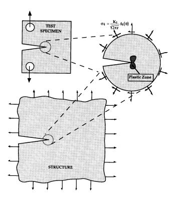
Figure 3-13 Schematic of crack-tip plasticity in test specimen and structure.
