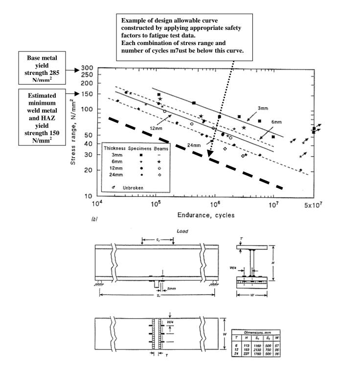
Figure 1-1 S/N curve for welded 6061-T6 Aluminum beam in bending
