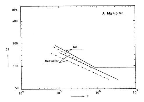
Figure E-5; T-Joint connection; Alloy AlMg4.5Mn; R = 0.1;
