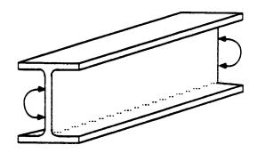
3.1(A) - EXTRUDED BEAM (FLEXURAL LOADING)
