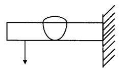
Figure 3-20 Small Specimen for 5383 Fatigue Tests
