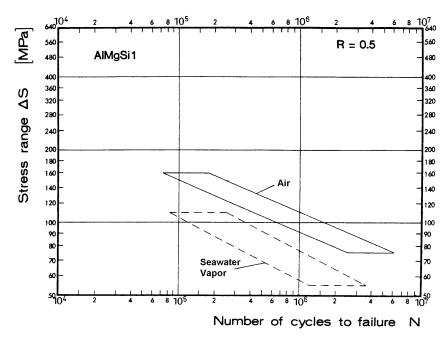
Figure E-7 Transversely welded plate; Alloy AlMgSi1; R = 0.5;
