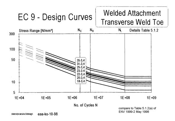
Fig. 5.2.2\* Design Curves  $\Delta \sigma$  - N for members with welded attachments / transverse weld toe detail categories in Table 5.1.2\*
