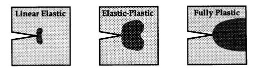
Figure 6-1 Relative Size of Plastic Zone at Crack Tip
