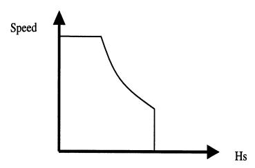
Figure 2-3 Speed/Wave Height Restriction Curve for High-Speed Craft
