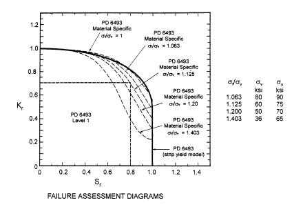
The Material Specific, FAC Curves represent: (1) elastic-perfectly plastic material, i.e.,  $\sigma_v/\sigma_v = 1$ , (2) A 36, i.e.,  $\sigma_v/\sigma_v = 1.403$ , (3) HSLA 50, i.e.,  $\sigma_v/\sigma_v = 1.200$  (4) HSLA 60, i.e.,  $\sigma_v/\sigma_v = 1.125$ , and (5) HSLA 80 i.e.,  $\sigma_v/\sigma_v = 1.063$ .
