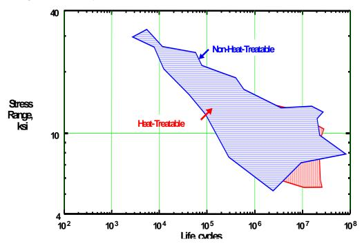
Figure 3-9 Axially Loaded, Transverse Butt-Welded 3/8 inch Aluminum Plate
