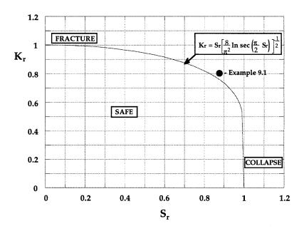
Figure 6-8 Typical Failure Assessment Diagram, FAD
