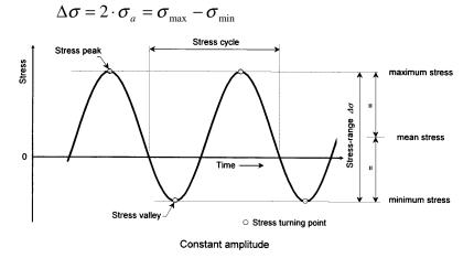
Figure 4-3 Constant Amplitude Curve
