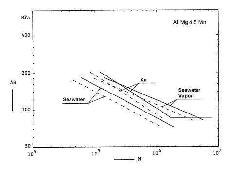
**Figure E-3; Transversely welded plate; Alloy AlMg4.5Mn; R = 0.1;**Error! Reference source not found.
