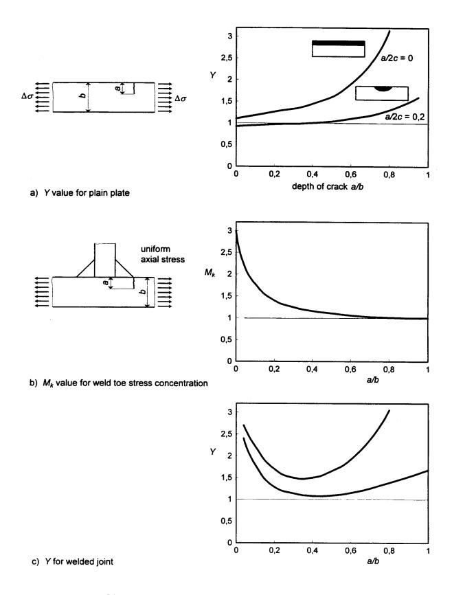
Figure B.4.1. Use of typical standard geometry solutions for y
