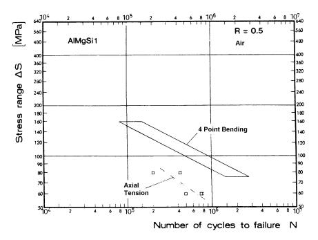
Figure E-15; T-Joint; Alloy AlMgSi1; R = 0.5;
