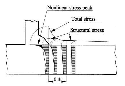
Figure 4-8 Local Stress Concentrations in Fillet Weld
