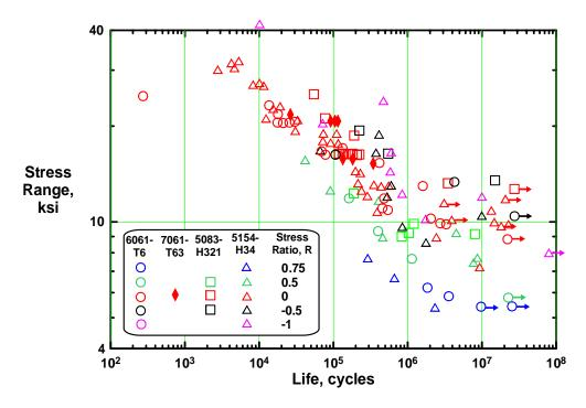
Figure 3-8 Axially Loaded, Transverse Butt-Welded 3/8 inch Aluminum Plate
