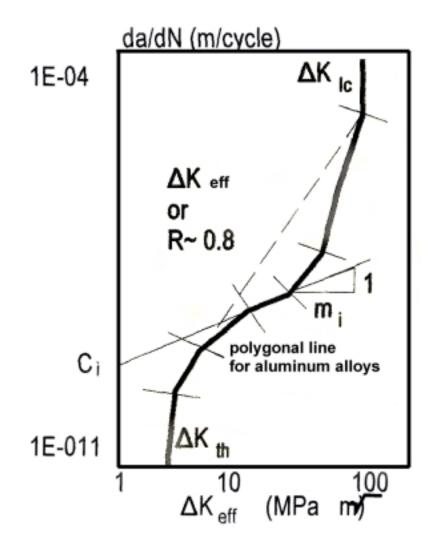
Figure 6-4 Polygonal da/dN curve for aluminum
