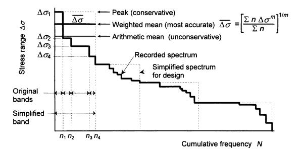
Figure 4.5.2. Simplified Stress Range Spectrum
