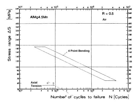
Figure E-14; T-Joint connection; Alloy AlMg4.5Mn; R = 0.5;
