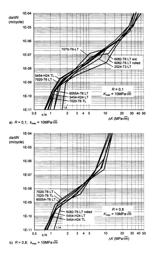
Figure B.3.5 Typical fatigue crack growth curves for various wrought alloys  $(K_{max}) = 10 \ MPa \ \sqrt{m}$
