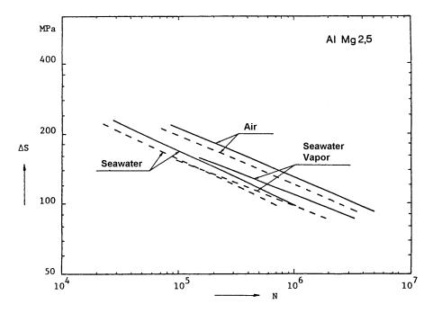
Figure E-4; Transversely welded plate; Alloy AlMg2.5; R-ratio = 0.1;
