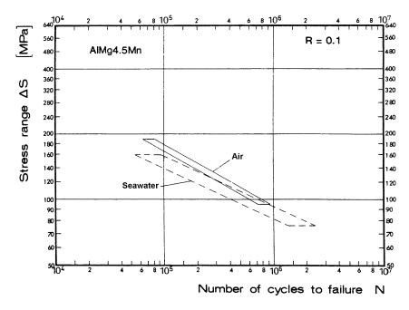
Figure E-8; T-Joint connection; Alloy 5083; R = 0.1;
