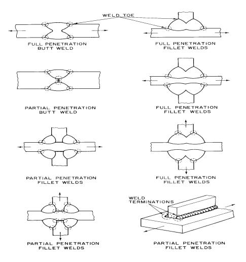
Figure 3-19 Stress Concentration Locations In Typical Welded Joints
