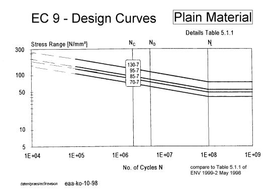
Fig. 5.2.1\* Design Curves  $\Delta \sigma$  - N for plain material detail categories in Table 5.1.1\*
