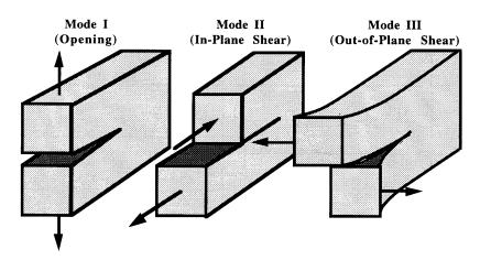
Figure 6-10 Three Modes of Loading for Crack Propagation
