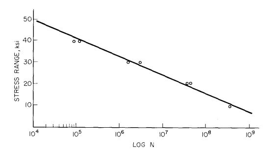
Figure 3-4 Long Life Fatigue for Aluminum
