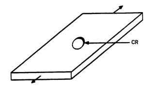
7.1.1(A) - PLATES WITH HOLES (AXIAL LOAD)
