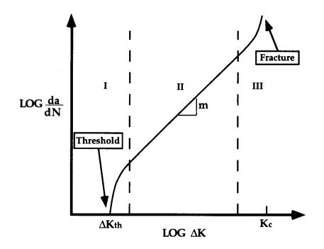
Figure 6-2 Typical FCGR Curve
