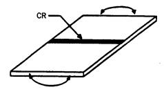
BUTT JOINTS — TRANSVERSE (FLEXURAL LOADING) 2.1.3(A) — WELD REINFORCEMENT INTACT
