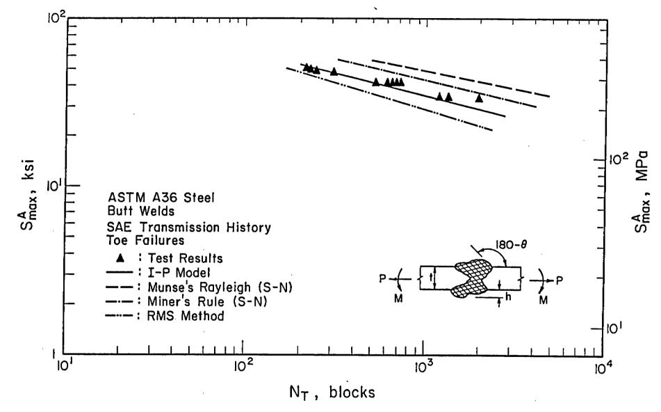
Fig. 2-4 Fatigue test results and predictions for ASTM A 36 butt welds subjected to SAE transmission history. SA is the maximum stress in the load history.
