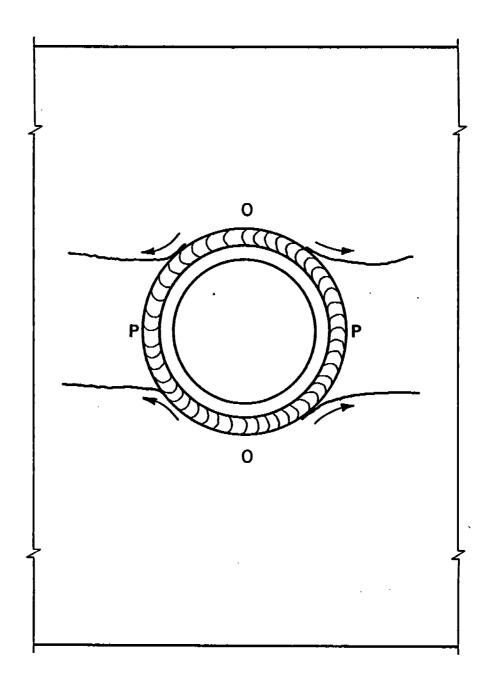
Fig. 5-26 Pattern of fatigue crack initiation and growth for detail no. 47. Fatigue cracks initiated at either of the two opposite locations mid-way between 0 and P and propagated through the plate normal to the principal stress.
