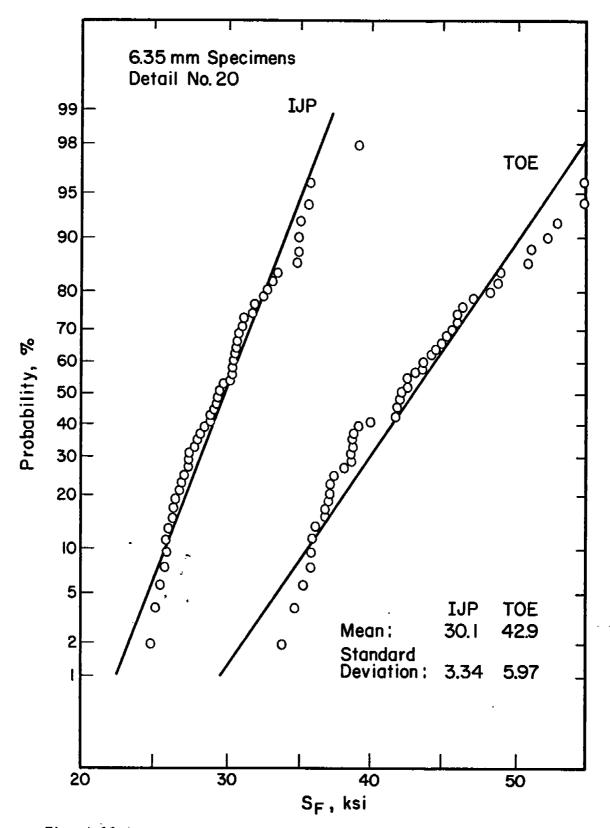
Fig. 4-13 A plot of the cumulative probability of the constant  $S_F$  for values of x (0 x 1) for 6.35 mm specimens. This simulates the situation in which the induced bending stresses can only increase or decrease the cyclic stress at some location in the weldment and hence only reduce the fatigue life.
