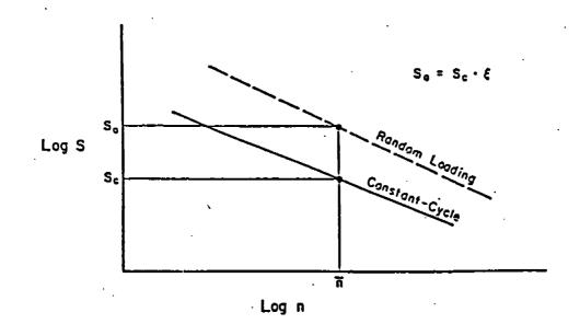
Fig. 1-7 Relationship between maximum stress range of variable (random) loading and equivalent constant-cycle stress range [1-4].
