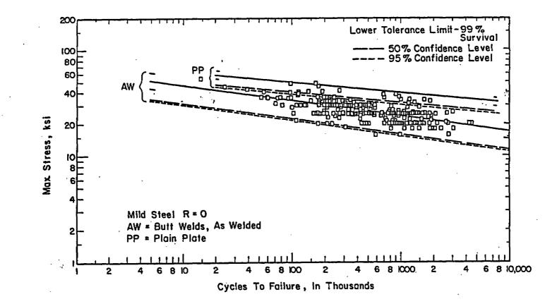
Fig. 1-2 Stress range versus cycle to failure for mild steel butt welds subjected to zero to tension loading. The fatigue resistance of as-welded butt weld is generally less than the fatigue resistance of plain plate which is also indicated in this figure [1-2].
