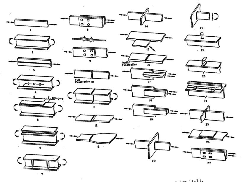
Fig. 1-1 Structural details provided in AISC fatigue provision [1-1].
