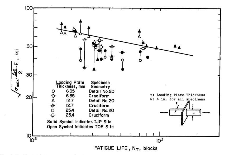
Fig. 3-21 The Smith-Watson-Topper (SWT) parameter versus total fatigue life in blocks. The SWT parameter reflects both the local mean stress and the range in local strain. The tie-lines connect the values of local mean stress for the IJP and toe of a given specimen in those cases in which both sites were active. The test-fit line is taken from Fig. 3-22.
