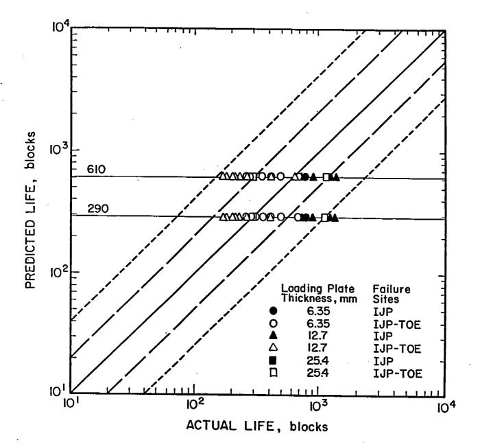
Fig. 4-2 Actual total fatigue lives (blocks) compared with total fatigue lives predicted using the Munse Fatigue Design Procedure. The top solid line is the prediction for the edited history. "The lower solid line is the prediction for the full SL-7 history. The dashed lines represent factors of two and four departures from perfect agreement.
