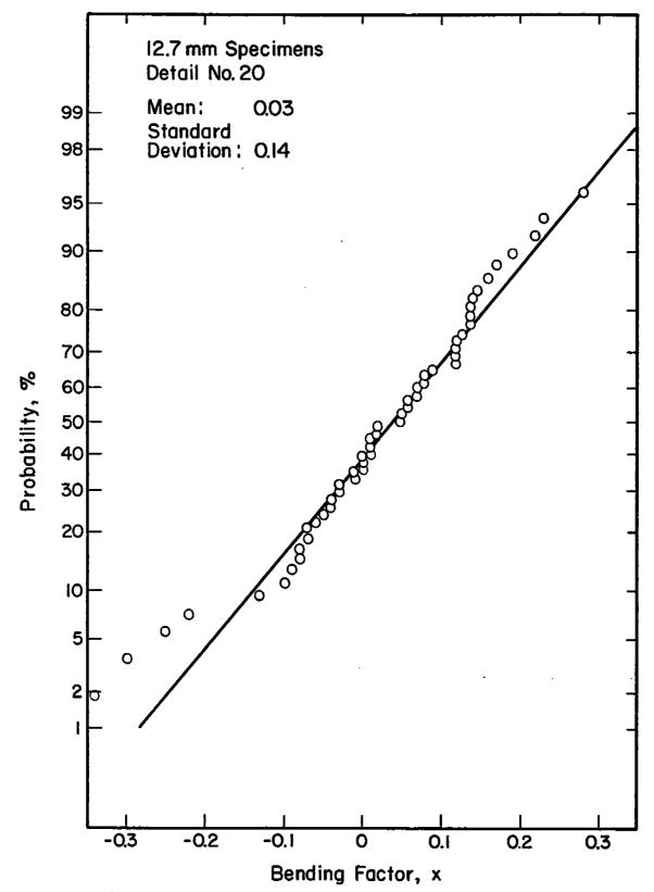
Fig. 4-9 A plot of the cumulative probability of the bending factor x on the normal probability paper which shows that x can be described by the normal probability distribution.
