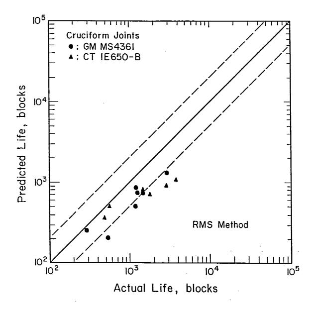
Fig. 2-9 Comparison of actual and predicted fatigue life using the RMS Method. The dashed lines represented factors of two departures from perfect agreement.
