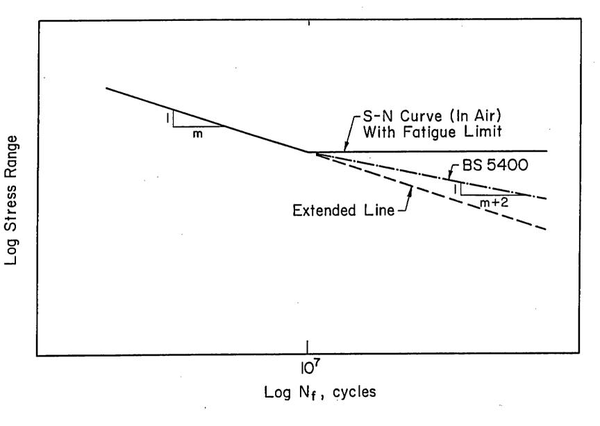
Fig. 2-1 Modification of S-N diagram.
