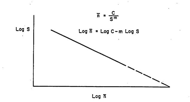
Fig. 1-3 Basic S-N relationship for fatigue [1-4].
