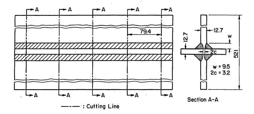
Fig. 3-12 Specimen details of cruciform joints for the study of mean stress effects. (Dimensions in mm.)
