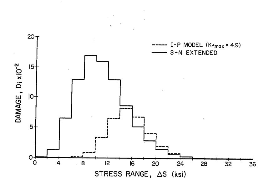
Fig. 3-4 Calculated damage attributable to each stress range interval for a Weibull distribution based on the 10<sup>8</sup> cycle SL-7 container ship history [1-4]. Damage was calculated using both the extended S-N curve and the I-P model as shown. The damage estimates depend upon the assumed shape of the S-N diagram in the high cycle region as well as the severity of the stress concentration K<sub>fmax</sub>: K<sub>fmax</sub> value was assumed as 4.9 at the IJP sites of Detail No. 20.
