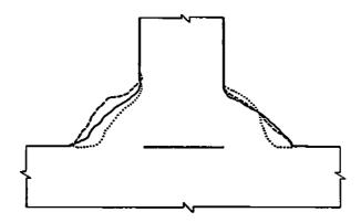
Schematic Comparison of the Actual Weld Configuration
