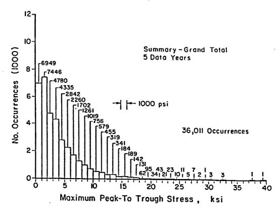
Fig. 3-1 Histogram from the SL-7 container ship scratch gauge data. The number of occurances during a five year history is plotted as a function of maximum peak-to-trough stress range [3-1].
