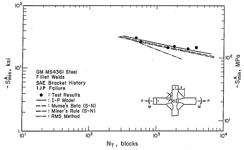
Fig. 2-2 Fatigue test results and predictions for GM MS4361 Fillet welded cruciform joints subjected to SAE Bracket history.  $S^A_{min}$  is the minimum stress in the load history. The Incomplete Joint penetration (IJP) is indicated by 2C.
