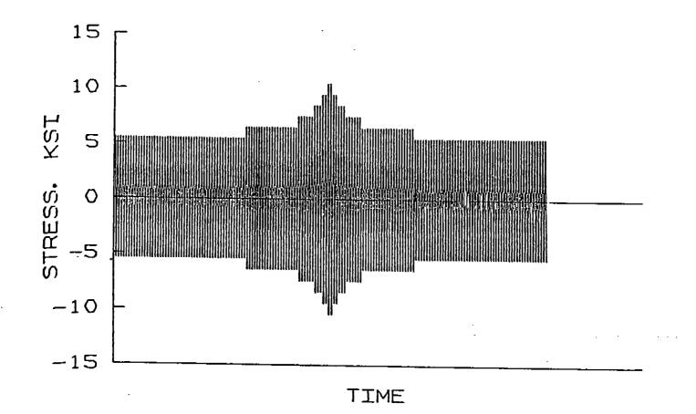
Fig. 3-6 Plot of one block of the constructed ship history having the 92.8% of the SL-7 container ship history damage. The central portion of the history represents a period of severe weather.
