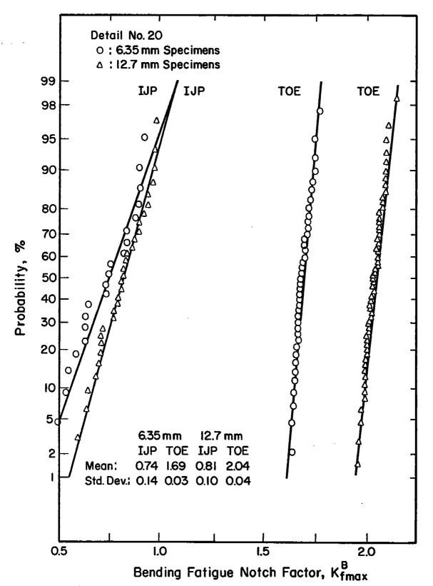
Fig. 4-8 A plot of the cumulative probability of the bending fatigue notch factor  $(K_{fmax}^B)$  on the normal probability paper which shows that the  $K_{fmax}^B$  can be described by the normal probability distribution.
