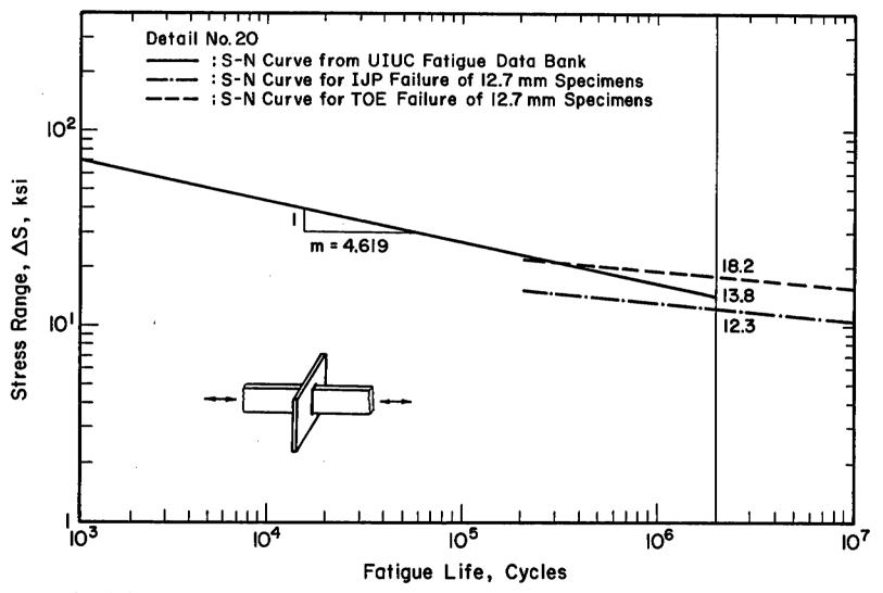
Fig. 4-6 Comparison of the S-N curve for detail No. 20 taken from the UIUC fatigue data bank with the long life behavior predicted by the I-P model. See Eq. 4-2.
