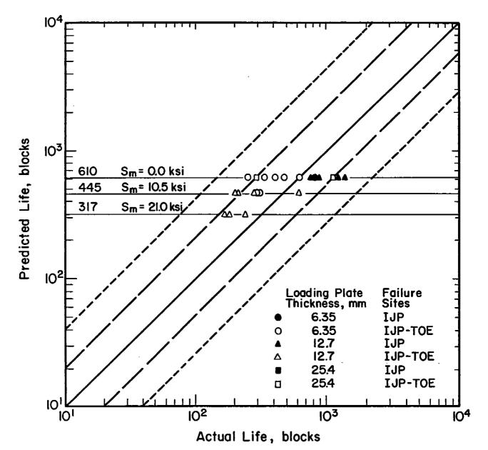
Fig. 4-3 Comparison of observed total lives with prediction of the Munse Fatigue Design Procedure modified to include the effects of mean stress. See Eq. 4-1. The horizontal solid lines are predictions for different levels of applied mean stress. The dashed line represent factors of two and four departures from perfect agreement.
