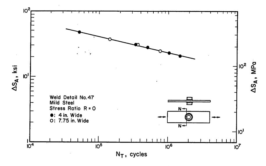
Fig. 5-25 Constant amplitude fatigue test results for detail no. 47. The net stress range was calculated at the section N-N.
