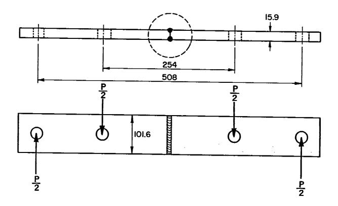
Fig. 5-13 Testpiece dimensions and loading conditions for detail no. 43 - a partial-penetration butt weld. (Dimensions in mm.)
