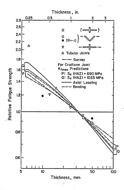
Fig. 3-23 Influence of plate thickness on fatigue Strength (normalized to a thickness of 32 mm, all tests at R=0 except where stated [3-6].
