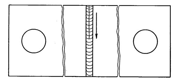
Fig. 5-16 Pattern of fatigue crack initiation and growth for detail no. 43. The fatigue crack initiated at the IJP of the extreme fiber of the specimen and propagated normal to the maximum principal stress.
