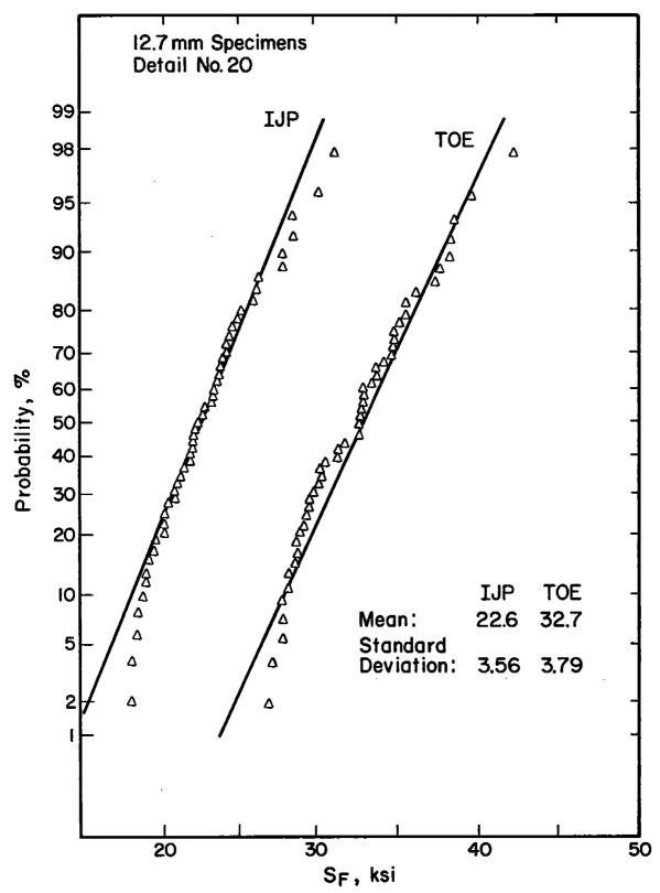
Fig. 4-10 A plot of the cumulative probability of the constant  $S_F$  for values of x (-1 x 1) for 12.7 mm specimens. This simulates the situation in which the bending stresses can only increase or decrease the cyclic stress and hence increase or decrease the fatigue life.
