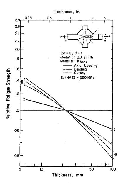
Fig. 3-24 The variation of predicted relative Fatigue strength with plate thickness (normalized to a thickness of 22 mm).
