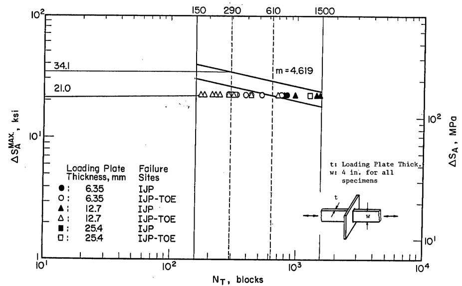
Fig. 4-1 Test data compared with the predictions of the Munse Fatigue Design Procedure. The sloped lower solid line is the prediction for the edited history. The sloped top solid line is the prediction for the full SL-7 history. The Munse Fatigue Design Procedure is based on the extended S-N diagram and therefore predicts a large influence for the small cycles absent in edited history. S<sub>A</sub><sup>max</sup> is the biggest stress range in the load history.
