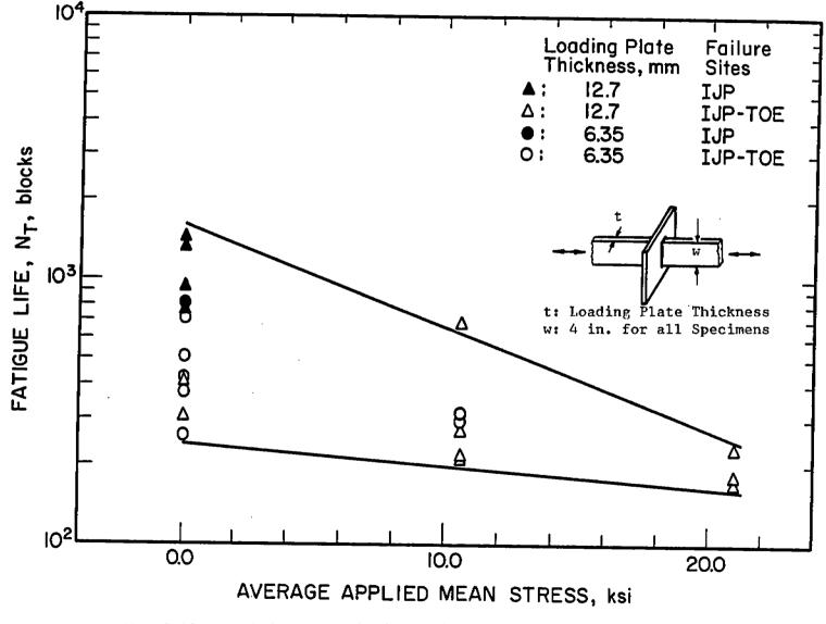
Fig. 3-18 Total fatigue life (blocks) versus the applied mean stress (ksi).
