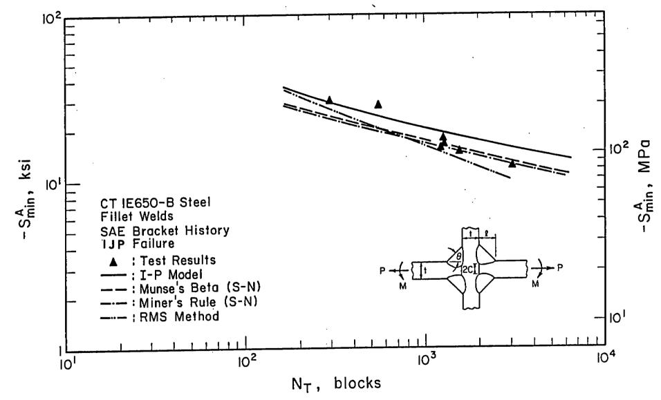
Fig. 2-3 Fatigue test results and predictions for CT 1E650-B fillet welded cruciform joints subjected to SAE Bracket history. SA is the minimum stress in the load history. The Incomplete Joint penetration (IJP) is indicated by 2C.
