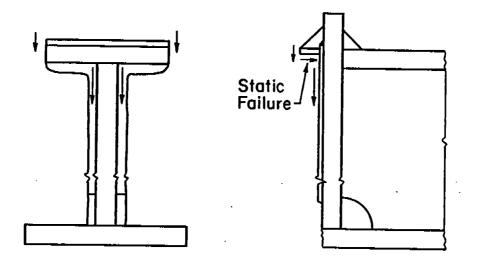
Fig. 5-11 A fatigue fracture surface and a schematic diagram of the failure mode of testpiece 39-A-4. The two fatigue crack initiation sites (one at the toe of the top flange plate, the other at the IJP of the fillet weld on the web) were connected by a shear failure. Testpieces 39-A-1 to 39-A-4 exhibited this type of behavior.
