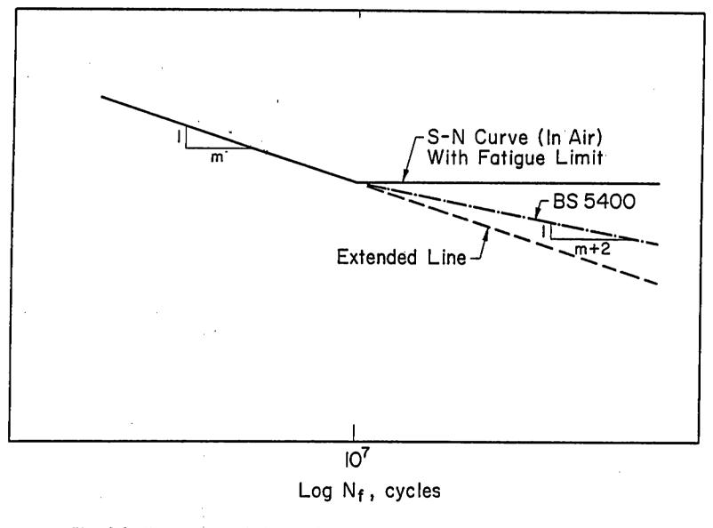
Fig. 3-3 Three suggested shapes of the S-N diagram in the long-life regieme.
