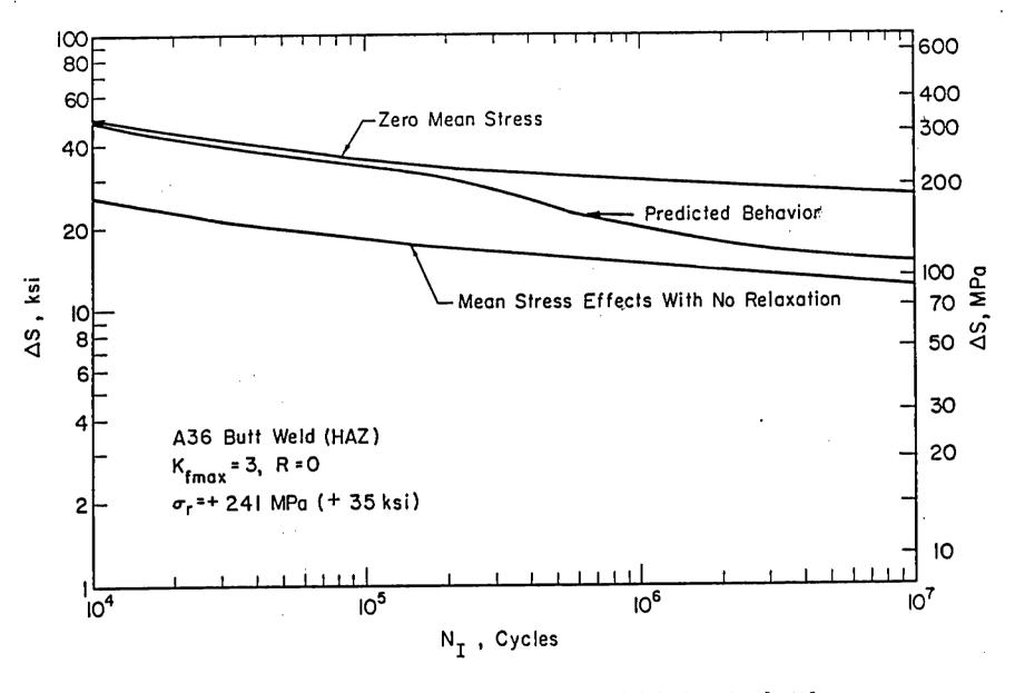
Fig. A-18 Mean stress relaxation influence on the fatigue crack initiation life [A-11].
