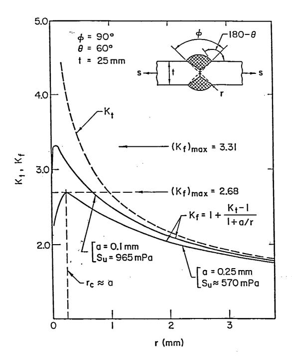
Fig. A-9 Elastic stress concentration factor  $(K_t)$  and fatigue notch factor  $(K_t)$  as a function of toe root radius.  $K_{fmax}$  is the "worst case" value of  $K_f$  for a given material and geometry.
