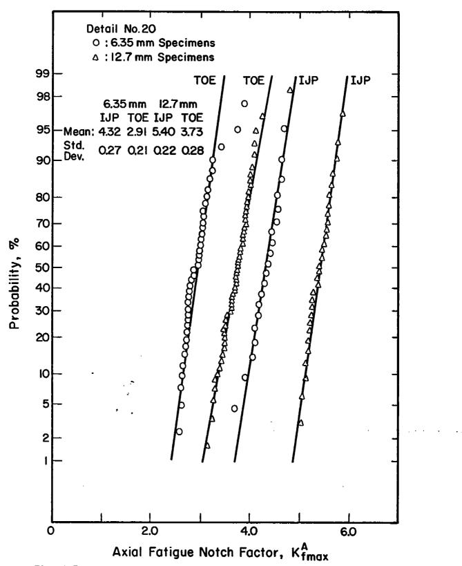
Fig. 4-7 A plot of the cumulative probability of the axial fatigue notch factor  $(K_{\rm fmax}^{\rm A})$  on the normal probability paper which shows that  $K_{\rm fmax}^{\rm A}$  is normally distributed.
