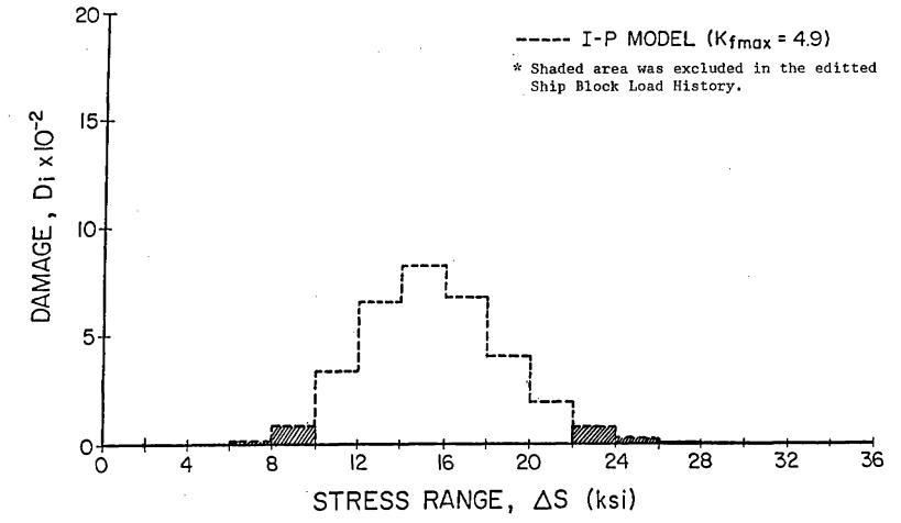
Fig. 3-5 Editing used to exclude unimportant small and large cycles. Stresses above 22 and below 10 ksi were excluded. The developed 5,047 cycle block represents 92.8% of the damage imparted during one month of the SL-7 ship history. K<sub>fmax</sub> value was assumed as 4.9 at the IJP sites of Detail No. 20.
