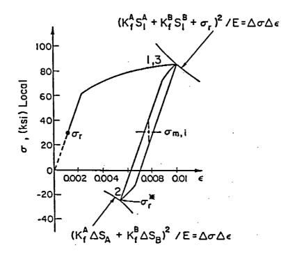
Fig. A-10 Set-up cycle analysis for the weld toe with tensile residual stresses. Note the change of the sign of the notchroot residual stresses after the second reversal of load.
