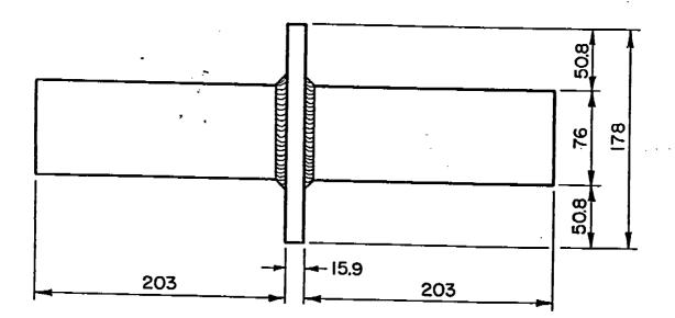
Fig. 3-9 Geometry and dimensions for testpieces of detail no. 20. (Dimensions in mm.)
