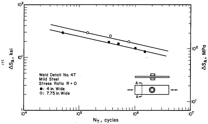
Fig. 5-24 Constant amplitude fatigue test results for detail no. 47. The nominal stress range was calculated at the section A-A.
