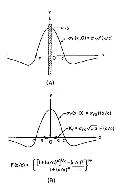
Fig. A-19 (a) Longitudinal residual stress field due to welding (hatched area: weld metal); (b) Crack in residual stress field [A-17].
