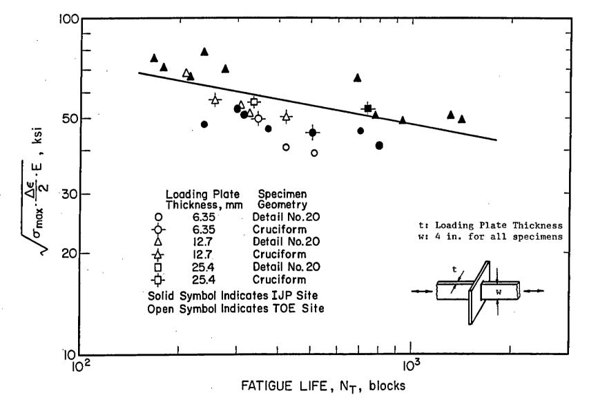
Fig. 3-22 The Smith-Watson-Topper (SWT) parameter versus total fatigue life in blocks. Only the location having the highest values of SWT parameter are plotted.
