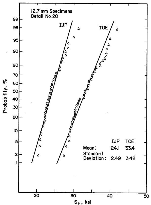
Fig. 4-11 A plot of the cumulative probability of the constant  $S_F$  for values of x (0 x 1) for 12.7 mm specimens. This simulates the situation in which the induced bending stresses can only increase or decrease the cyclic stress at some location in the weldment and hence only reduce the fatigue life.
