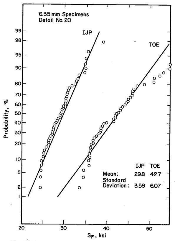
Fig. 4-12 A plot of the cumulative probability of the constant  $S_F$  for values of x (-1 x 1) for 6.35 mm specimens. This simulates the situation in which the induced bending stresses can either increase or decrease the cyclic stress and hence increase or reduce the fatigue life.
