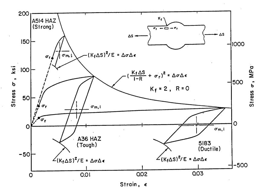
Fig. A-11 Set-up cycle for ASTM A514 HAZ (strong), A36 HAZ (tough) steels, and aluminum alloy 5183 WM (ductile) materials [A-11]. The set-up cycle may eliminate notch-root residual stresses in ductile materials.
