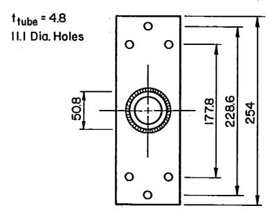
Fig. 5-17 Testpiece dimensions and loading conditions for detail no. 44 --- a tubular cantilever beam. (Dimensions in mm.)
