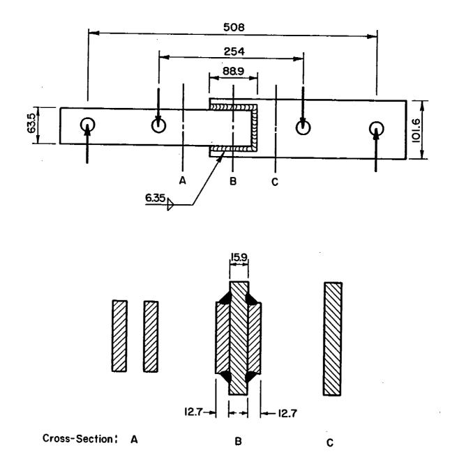
Fig. 5-2 Testpiece dimensions and loading conditions for detail no. 34--a fillet welded lap joint. (Dimensions in mm.)
