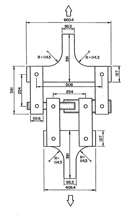
Fig. 5-3 Loading fixture design for detail no. 34. (Dimensions in mm.)
