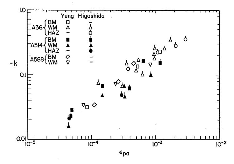
Fig. A-6 Relaxation exponent as a function of plastic strain amplitude [A-1, A-8].
