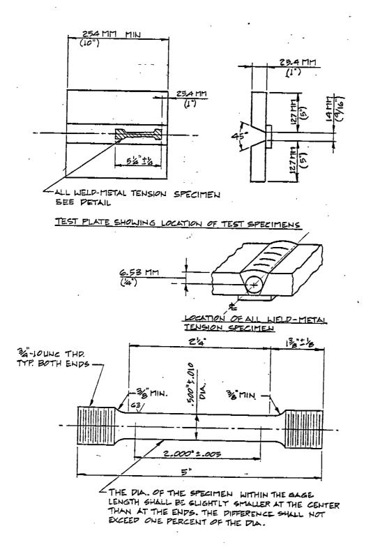
FIGURE A-11 LOCATION AND DRAWING OF ALL-WELD-METAL TENSILE TEST SPECIMEN
