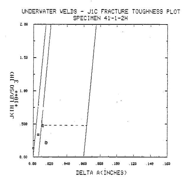
FIGURE A-17 J-RESISTANCE CURVE: SPECIMEN 41-1-2H
