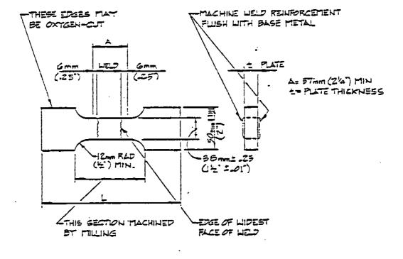
FIGURE A-5 TRANSVERSE-WELD REDUCED-SECTION TENSILE TEST SPECIMEN
