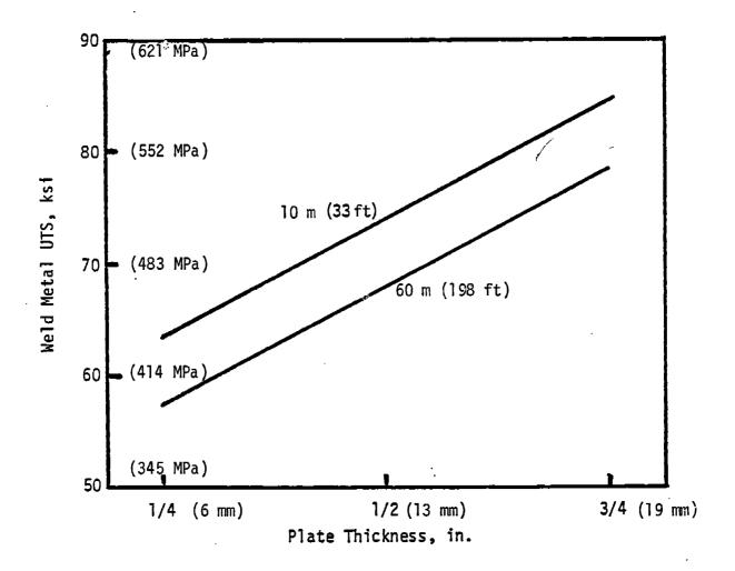
FIGURE 2.4. EFFECT OF PLATE THICKNESS AND WELDING DEPTH ON WELD METAL TENSILE STRENGTH.
