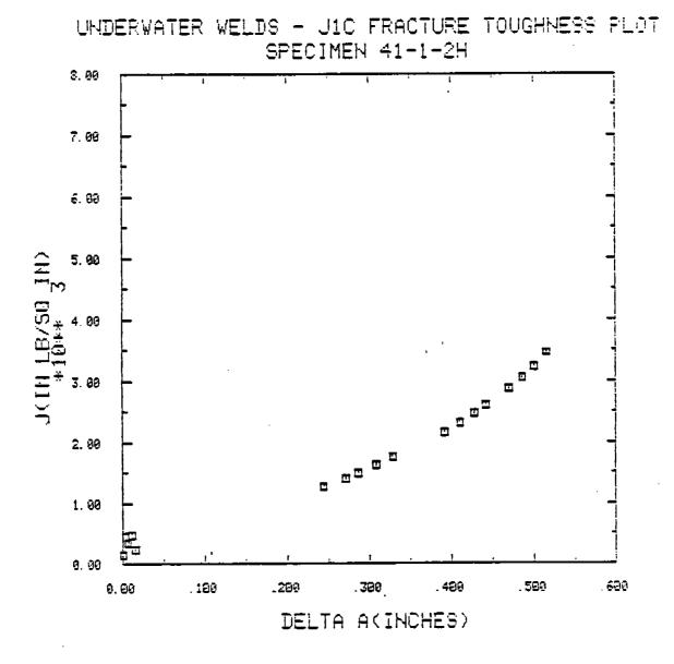
FIGURE A-16 FULL RANGE J-RESISTANCE CURVE: SPECIMEN 41-1-2H Note: 1.0 in. = 25.4 mm 1.0 in-1b/in<sup>2</sup> = 0.175  $\frac{kJ}{m^2}$
