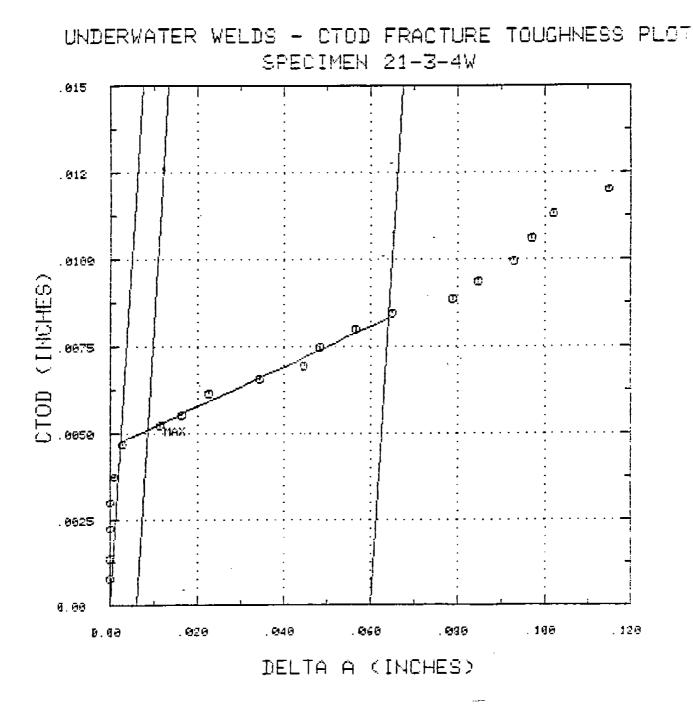
FIGURE 3.4. EXAMPLE OF CTOD RESISTANCE CURVE 1.0 in. = 25.4 mm
