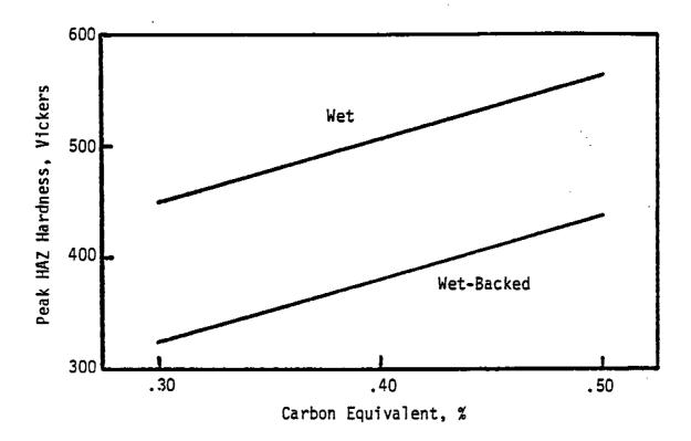
FIGURE 2.3. EFFECT OF CARBON EQUIVALENT AND WET VS WET-BACKED WELDING ON HAZ HARDNESS.
