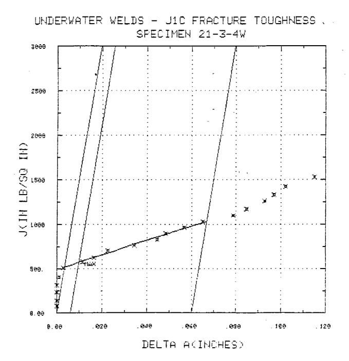
FIGURE 3.3 EXAMPLE OF J RESISTANCE CURVE
