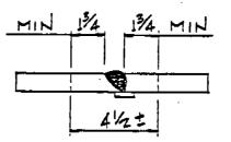
B SAW CUT A NOMINAL 41/2" LENGTH OF THE STRIP W/BOTH CUTS AT LEAST 13/4" FROM THE WELD CROWN
