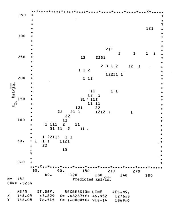
FIGURE 4.8. RESULTS OF REGRESSION ANALYSIS:  $K_{Ic}$  VS  $K_{Ic}$  PREDICTED BY RELATION (h) WHICH INCLUDES CVN AS WELL AS MATERIAL, DEPTH, ZONE, AND RESTRAINT FOR ALL TEST DATA ON UNDERWATER WELDS
