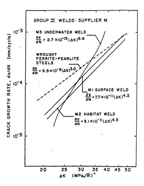
FIGURE 2.1. SIGMOIDAL SHAPE OF CRACK GROWTH RATE CURVE FOR UNDERWATER WELD WITH POROSITY [REF. 2.10].
