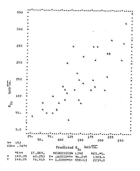
FIGURE 4.6. RESULTS OF REGRESSION ANALYSIS: K<sub>Ic</sub> VS PREDICTED BY RELATION (g) AS A FUNCTION OF MATERIAL, THICKNESS, DEPTH, ZONE, AND RESTRAINT FOR ALL TEST DATA ON UNDERWATER WELDS
