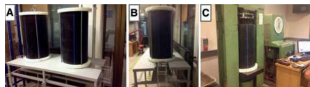
Figure 3—Lateral (A) and front view (B) of the laboratory model, and sample compression by hydraulic press (C)
