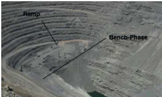
Figure 1—Phase benches and access ramps in an open-pit mine
