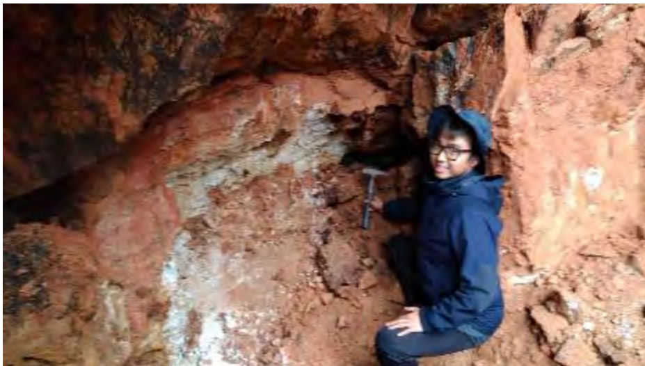
Figure 10.3: The Digging Face of the Main Inclined Shaft at Gubong showing clay fill to be removed.
