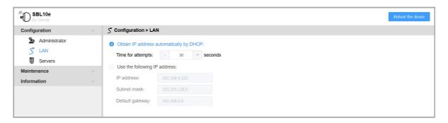
■ By default, the device is configured with DHCP activated. In case the DHCP server is not available, after the DHCP timeout, the device ends up using the static IP address whose default value is 192.168.0.2 when it has not been changed yet by the end user.
