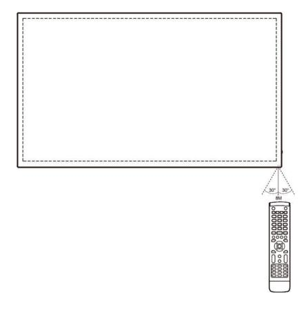
Remote control can work normally within the range of 8 meters, 30 degrees left and right from the remote-control receiver.
