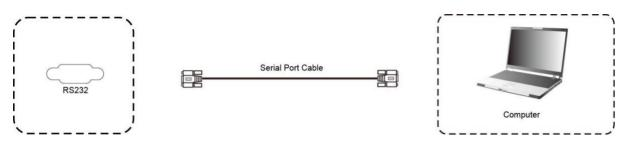
After using the serial port cable to connect central control equipment and the product, certain functions of the product can be controlled via the central control equipment, such as: power ON/OFF, sound volume adjustment, etc.
