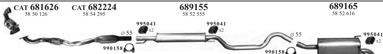
Zafira B 1.9CDTi-16v MPV 07'2005- Eng.Z1.9DTL 1910cc 74kW-101hp, Eng.Z1.9DT 1910cc 88kW-120hp, Z1.9DTH 1910cc 110kW-150hp Type A05
