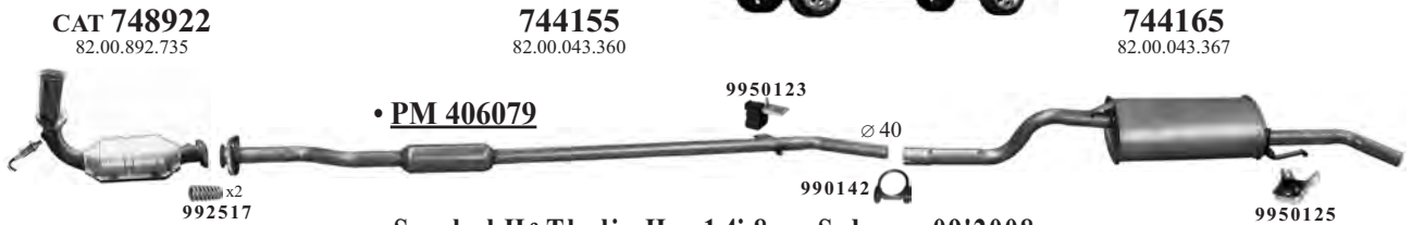
Symbol II & Thalia II 1.4i-8v Sedan 09'2008- Eng.K7J700, K7J718 1390cc 55kW-75hp Symbol Type LUK3, Thalia Type LBOB, LB17
