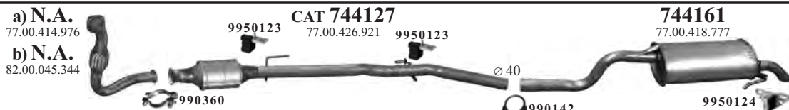
Clio II 1.9-8v Diesel Hatchback 03'1998-12'2002 Eng.F8Q 1870cc 48kW-65hp a) -04'2000, b) 05'2000- Type BB, CB, SB
