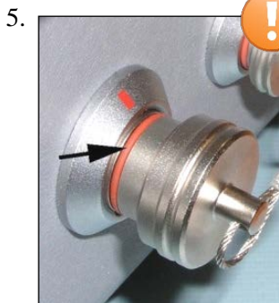
Connector protective cap – not properly inserted in connector (o-ring still visible).
