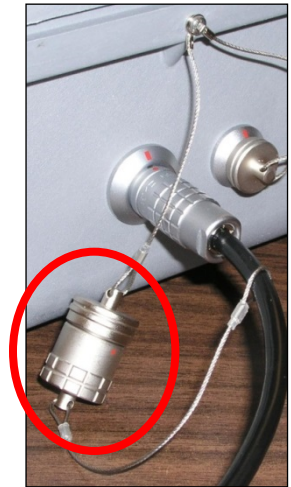
Join protective caps when they're not in use.
