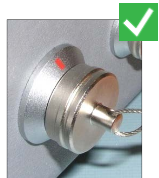
Connector protective cap – properly inserted in connector.
