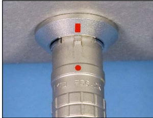
Connector properly lined up.
